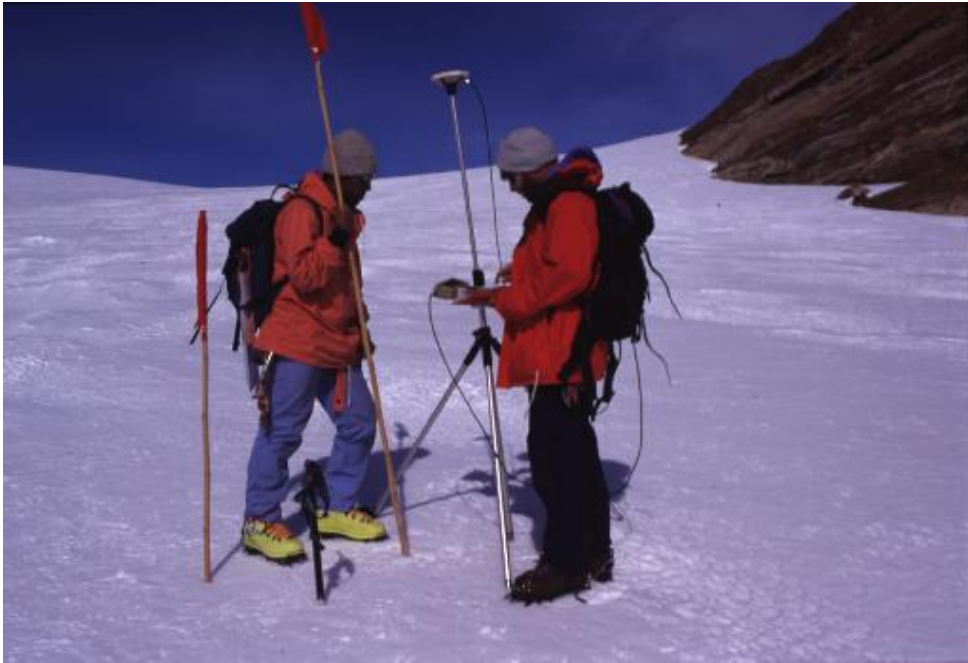
Figure 1: Monitoring ice movement by measuring bamboo stakes with differential GPS on Heito Glacier, Antarctica, during the 41st Japanese Antarctic Research Expedition.
