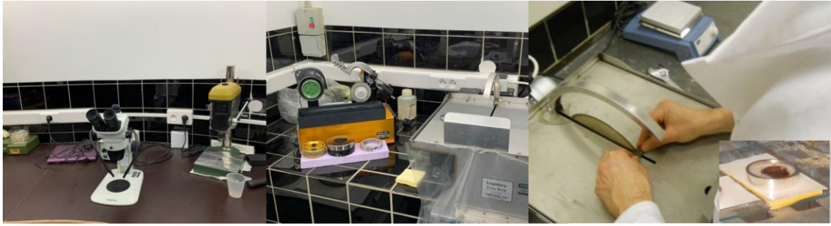
Figure 4. Detailed photos of the Proxxon drilling device and of the saws. A polished section of a meteorite is also illustrated.
