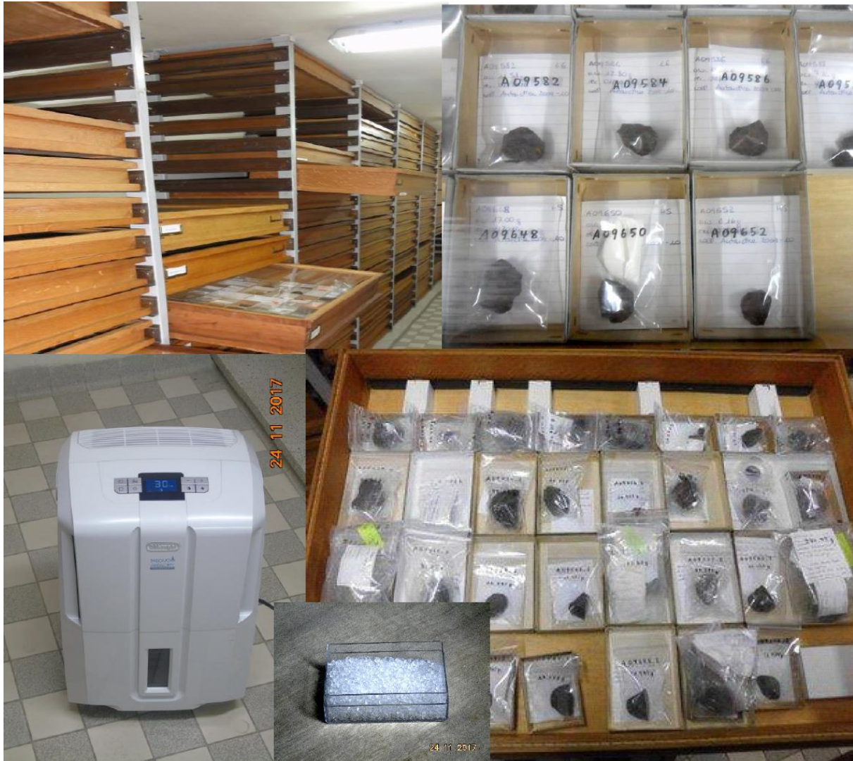
Figure 2. Photos of (i) the repository at the RBINS, (ii) the samples classified in the drawers, (iii) the silicagel used in order to prevent humidity in the drawers, and (iv) the dehumidifier that has been installed in the room.
