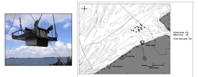
Figure 5. Positions of Semi-Grab (photo), Box-Core and Van Veen grab samples acquired during Belgica cruise 2009-29 (October 2009).
