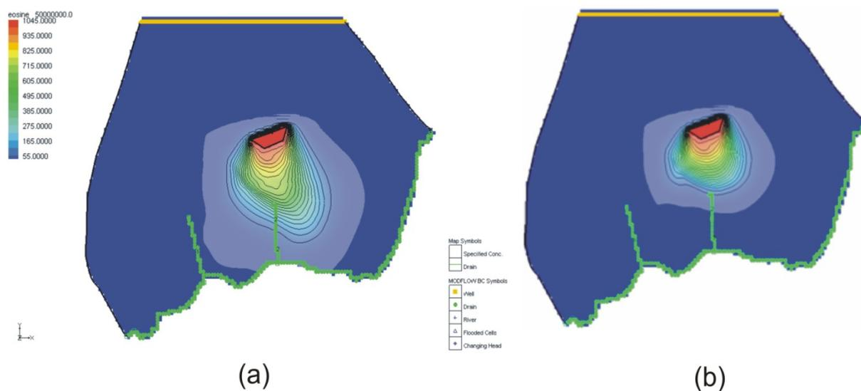
Figure 8: (a) Dispersion and advection, (b) Dispersion, advection and adsorption
