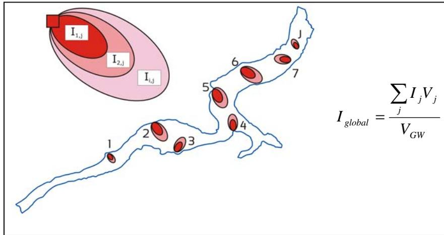
Figure 16: Risk assessment indicators defined for the source of contaminant on the groundwater body RWM073.
