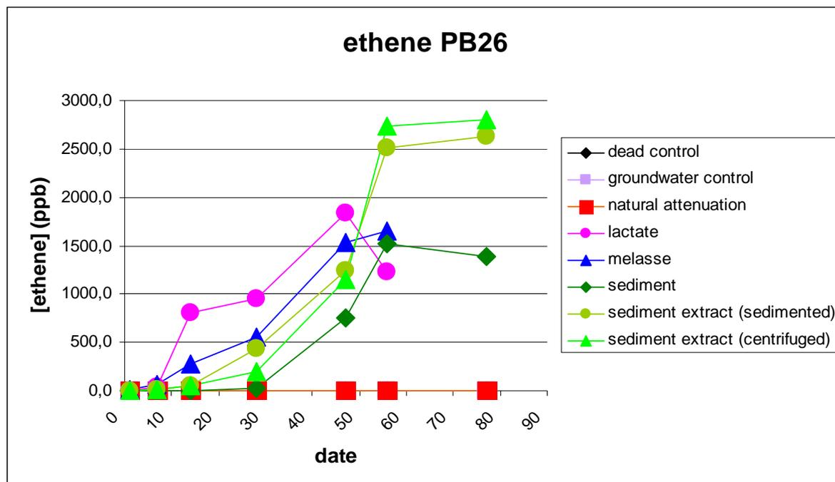
Figure 10: (Stimulated) degradation of DCE and subsequently VC to ethene at the location Pb 26 at the Vilvoorde-Machelen site.
