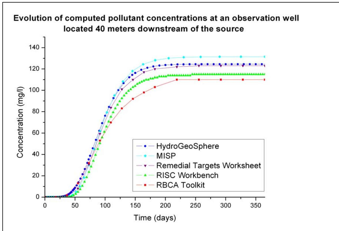
Figure 14: Evolution of contaminant concentrations “analytical vs numerical models”
