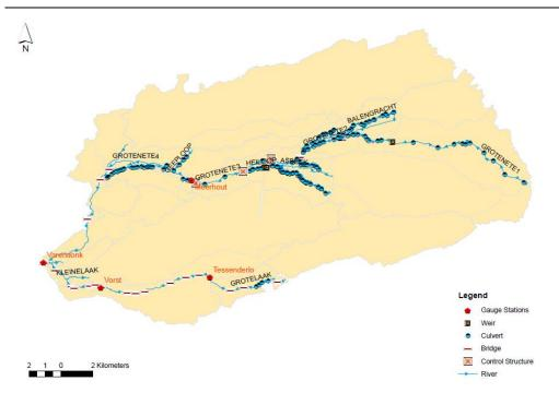
Figure 47. Overlay of the river hydraulic model on the Grote Nete river network.
