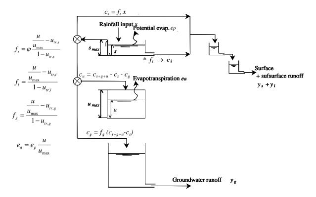
Figure 37. Model-structure of the NAM lumped conceptual rainfall-runoff model.
