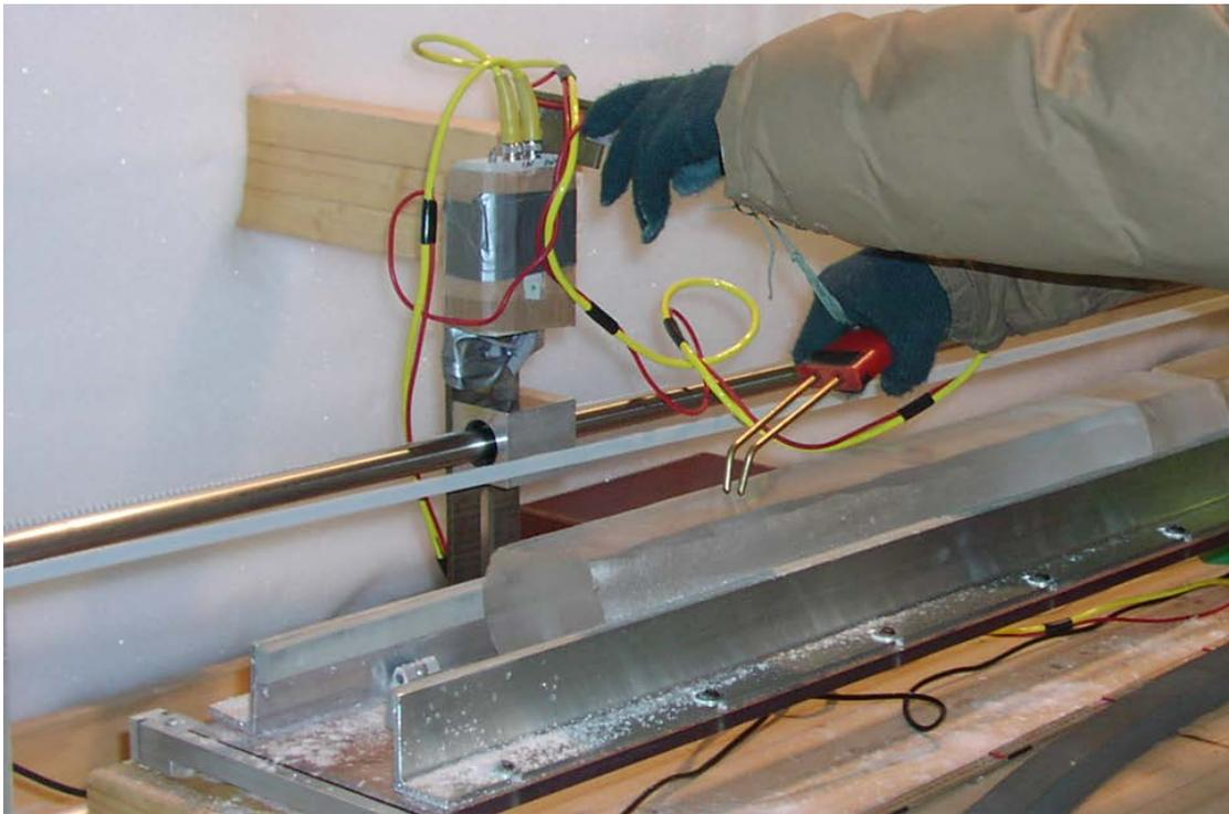
**Fig. 2.3.3 :** ECM measurement on an ice core
