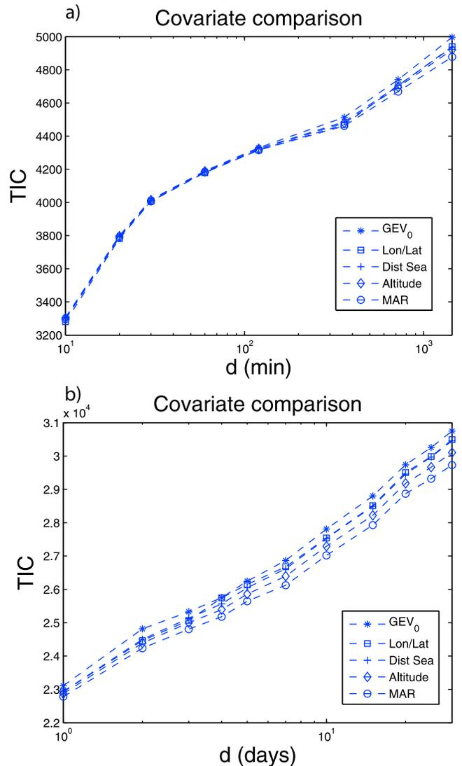
**Figure 5.** TIC against rainfall duration. Covariates for location parameter. (a) Short durations 10–1440 min. (b) Long durations 1–30 days.
