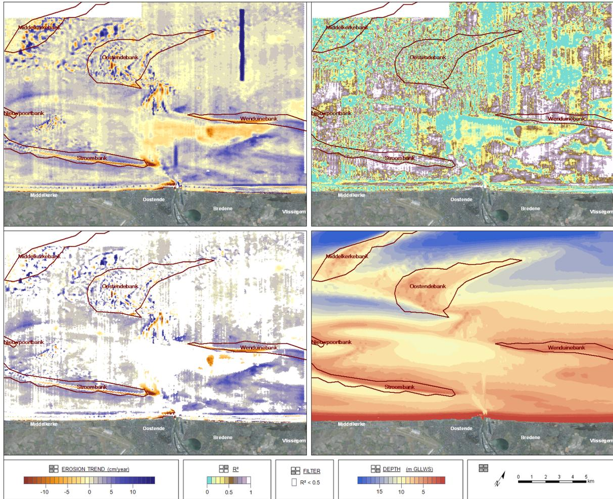
Figure A2-12. Erosion and sedimentation trends for coastal region between Westende and De Haan.
