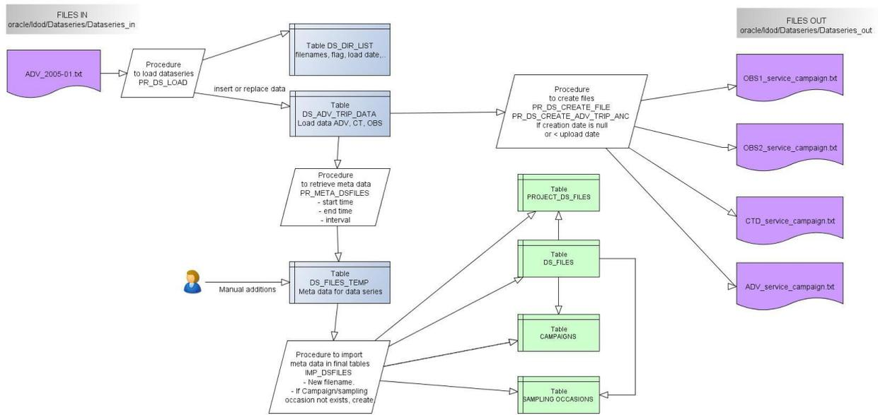
Figure A1-2: Import/export flow for ADV, CTD and OBS data from tripod moorings.
