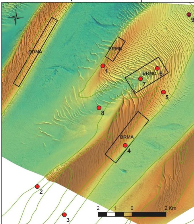
Figure A6-4. Buiten Ratel locations for sediment transport evaluation. Multibeam bathymetry from FPS Economy, SME's, Self-Employed and Energy, Marine Sand Fund. The black boxes indicate the monitoring areas (BRMA, BRMB, BRMC).
