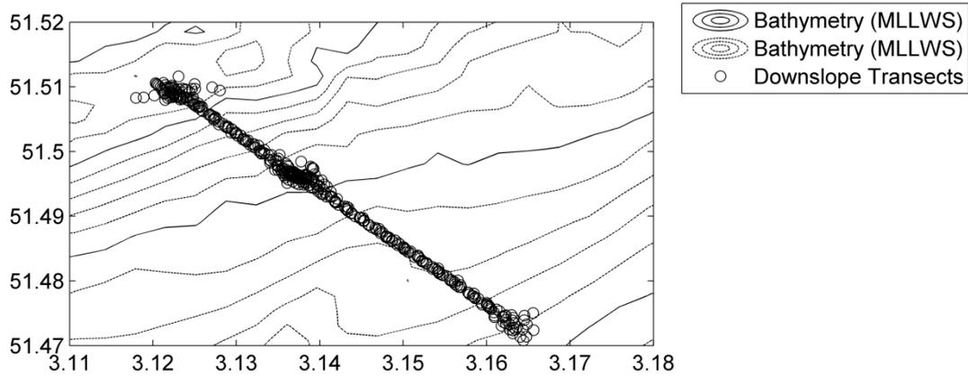
Figure A3-5. ADCP transects (upslope & downslope) over a 13-hrs period. Vertical profiling of turbidity, CTD and in-situ particle size (LISST) was carried out at a slope (midway) and gully position (north).
