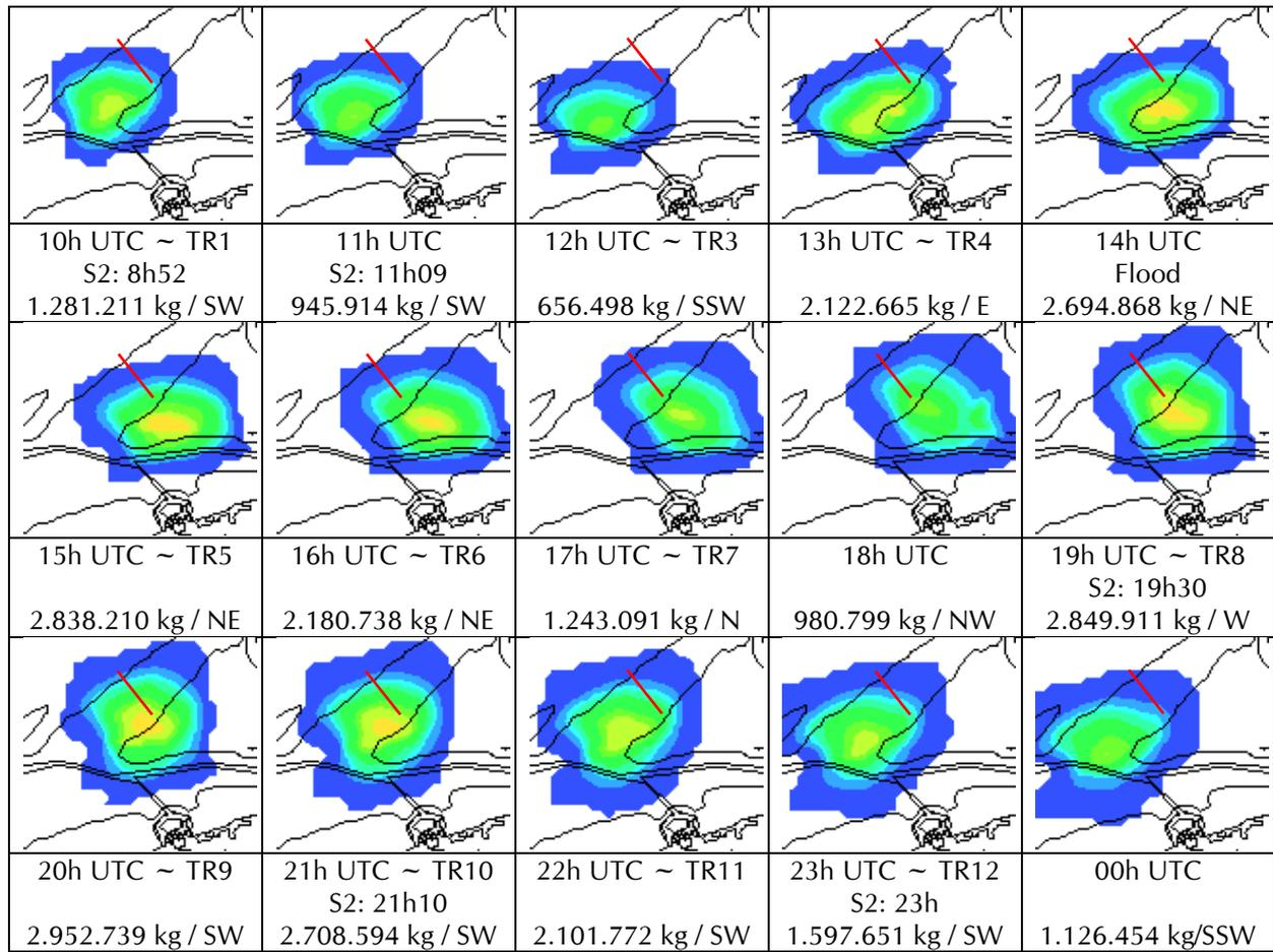
Figure A3-15. Modelled influence area of consecutive disposal of dredged material at the S2 disposal ground, period 22/3/11 10h to 23/3/11 00h. Eleven disposal activities were accounted for, starting on 21/3/11 8h32 and ending on 22/3/11 22h59. The timing of disposal events at the S2 location is given, as also the total mass (kg) and the direction of the current. Equinox conditions. On the ADCP transects (red line) a turbidity plume was observed from 17-21h UTC.
