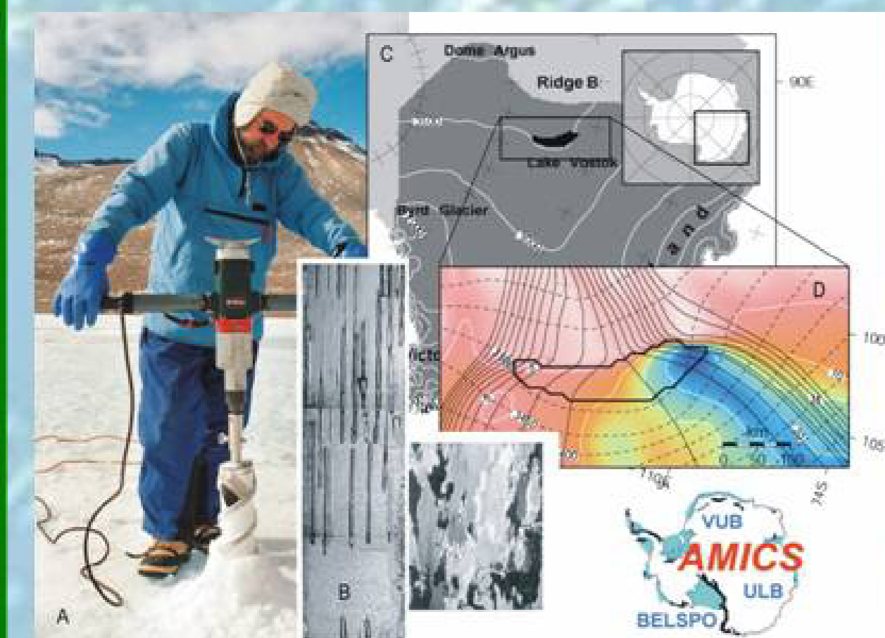
Fig.1.(A) Ice coring from the surface of Lake Victoria Upper (Victoria Valley, Antarctica); (B) Different vertical sections cut in a lake ice core: vertical cylindrical bubbles (left) and elongated crystals with irregular boundaries (right). Other parameter investigated are ionic and isotopic composition, gas content and composition; (C+D): dynamic interaction between the ice sheet and a subglacial lake leads to an anomaly in ice flow due to the reduced friction. Lake Vostok (shown here) thus forms a potential onset (blue area) of fast and/or enhanced ice flow deep in the interior of the Antarctic ice sheet
