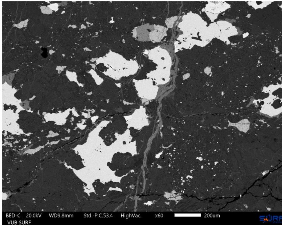
**Figure 4.** Scanning Electron Backscattered image of a representative area of A10177, showing the extent of terrestrial weathering in the Antarctic environment. White areas represent elements with a high Z-contrast, that is FeNi metal; dark grey areas represent elements with a low Z-contrast, that are silicate phases; light grey represent iron oxide rims around FeNi metal grains or oxide veins.
