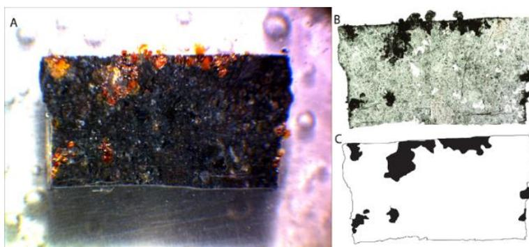
**Figure 8.** Extent of weathering after the cycle 2 on MET-3. A) Optical image of the weathering products, which are evidenced by a red-brownish colour, typical of rust. B) Reflected light image of the sample, allowing a clear identification of the rough weathering product (C)
