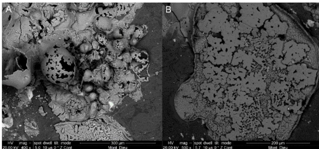
Figure 13. “Incomplete” shelled structures on MET-3.
