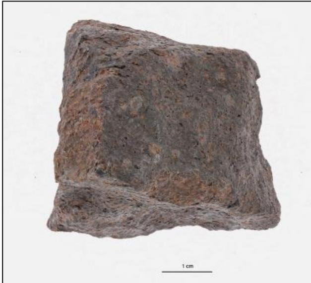
**Figure 2. Photograph of the external surface of the sample of A10177 held at the RBINS. The black area corresponds to the fusion crust that has not flaked off. Brownish red patches correspond to “metallic rust”, that is a common product of terrestrial alteration of FeNi metal in Antarctic meteorites (Bland et al., 2006; Gooding, 1986).**
