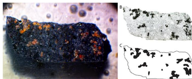
**Figure 10.** Extent of weathering after the cycle 4 on MET-5. For A, B and C, refer to figure 8 caption.
