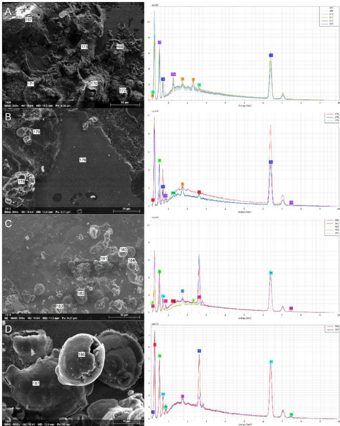
**Figure 15. Secondary Electron images of areas of EDS analyses of weathering products in MET-3 (A) and MET- 5 (B, C and D) and corresponding EDS spectra.**
