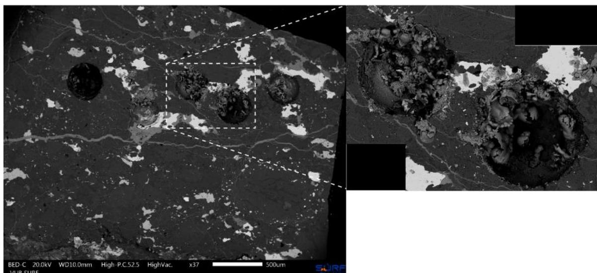
**Figure 7. Scanning electron backscattered image of a drill cavity in MET-2 after the second cycle of weathering. Abundant tubular overgrowths are in the cavity, which consist essentially of iron oxide with Cl detectable with EDS.**
