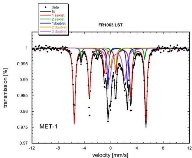
Figure 19. Mössbauer spectra (black line) of MET-1 powder. Several sextet and doublets are identified. Red sextet is identified as kamacite; Green sextet is identified as an Iron Sulphur (probably troilite); Blue and lavender doublets are identified as olivine and pyroxene, respectively; finally, brown doublet is difficult to identify and may be ferrihydrite.
