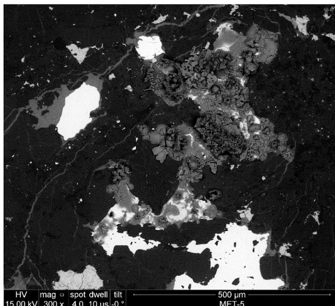
**Figure 11. Scanning electron image of a weathered area of MET-5 showing that at an early-stage weathering products are associated with FeNi metal.**
