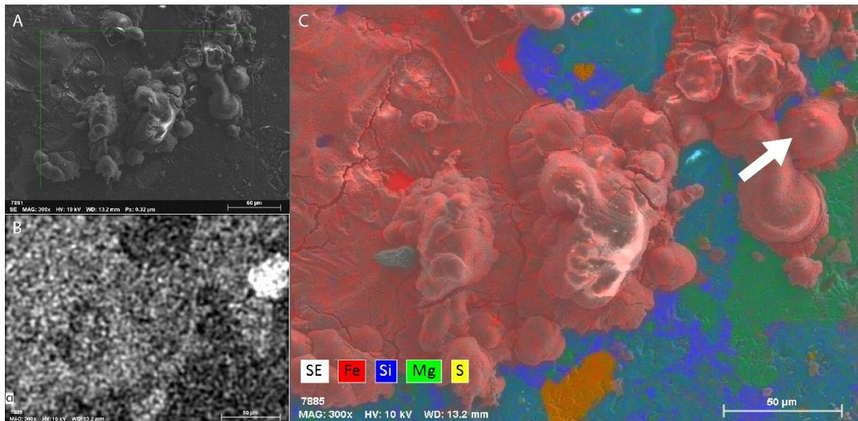
**Figure 16. Major element map of weathering products of MET-3. A) Secondary Electron image of the area of analysis. B) Chlorine is detected in all products, but only rare “hot spots” are observed. C) Composite image showing that weathering products are essentially composed of iron. Blue, green and orange areas correspond to pyroxene, olivine and troilite, respectively.**
