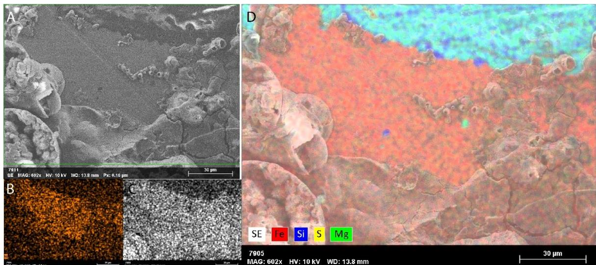
**Figure 17. Major element map of weathering products of MET-4. A) Secondary Electron image of the area of analysis. B) Weathering products are rich in Ni. C) Chlorine is virtually absent from weathering products in this sample. D) Composite image showing that weathering products are essentially composed of iron. Blue and red areas correspond to olivine and FeNi metal, respectively.**
