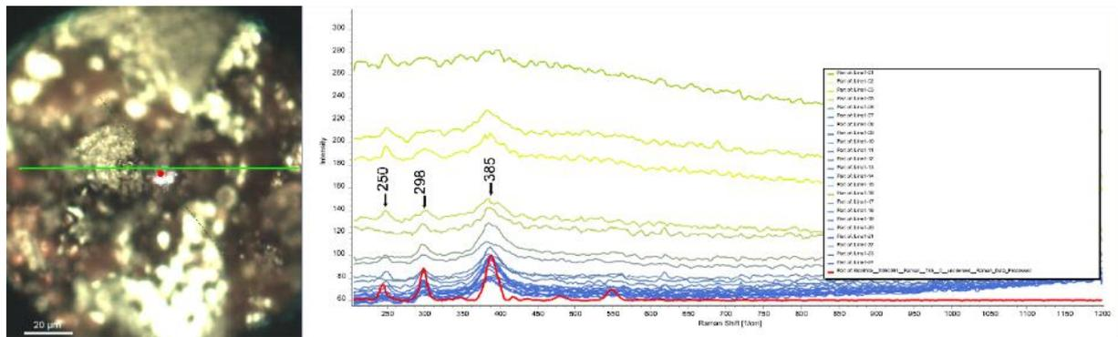
Figure 22. Raman spectra of weathering products in MET-4. Line (green on optical image) analyses showing good matches with goethite (red line; RRUFF ID: X050091).
