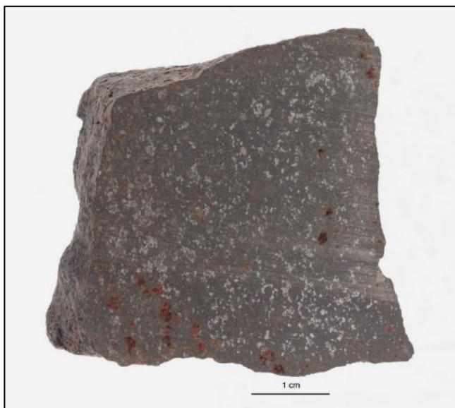
**Figure 3. Photograph of the sectioned side of A10177, exhibiting its interior. The brownish areas near the edge of the sample correspond to weathered FeNi metal grains to limonite. In the most severe cases, the metal dissolved entirely, leaving cavities partially filled with weathering products. However, light grey areas correspond to pristine FeNi metal grains and/or troilite, showing that the interior of the meteorite is mostly unweathered.**
