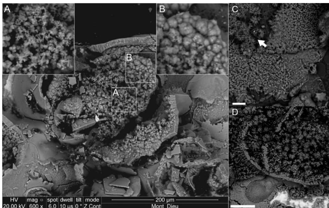
Figure 14. Scanning backscattered image of a “collapsed” shelled structure on MET-3. A) The material in the inner part of the structure show “cigar-shaped” crystals, typical of akaganeite; B) “globular” structures typical of goethite; C) Arrowed are “cotton-ball” crystals typical of akaganeite above an area of “fine plates” crystals typical of lepidocrocite; D) The interior of some shelled structures is exclusively constituted of “cotton-ball” crystals typical of akaganeite.
