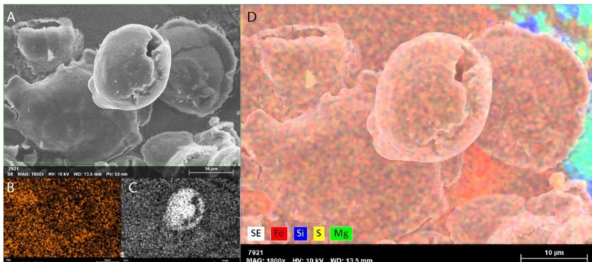
**Figure 18. Major element map of weathering products of MET-5. A) Secondary Electron image of the area of analysis. B) Nickel map. B) Tubular structures are usually richer in Cl than surrounding phases. D) Composite image showing that weathering products are essentially composed of iron. Blue, green and red areas correspond to pyroxene, olivine and FeNi metal, respectively.**
