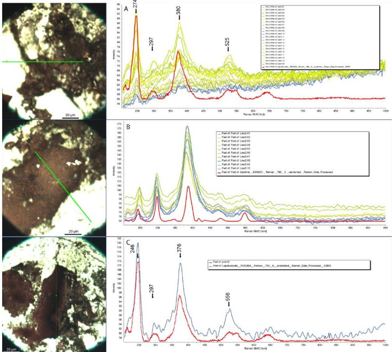
Figure 23. Raman spectra of weathering products in MET-5. A and B are line analyses (green lines on optical images) and C a point analysis (green point). A and B) most weathering products show a match with the spectrum of lepidocrocite (red line; RRUFF ID: R050554). C) some weathering products show a match with goethite (red line; RRUFF ID: X050091). Note: spectra of FeNi metal were not displayed.
