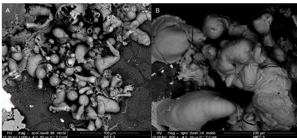
**Figure 12. Scanning electron backscattered image of tubular weathering products on the surface of MET-3 and MET-4.**
