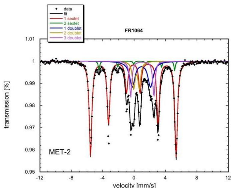
Figure 20. Mössbauer spectra (black line) of MET-2 powder. Peaks are identical as those observed in MET-1.
