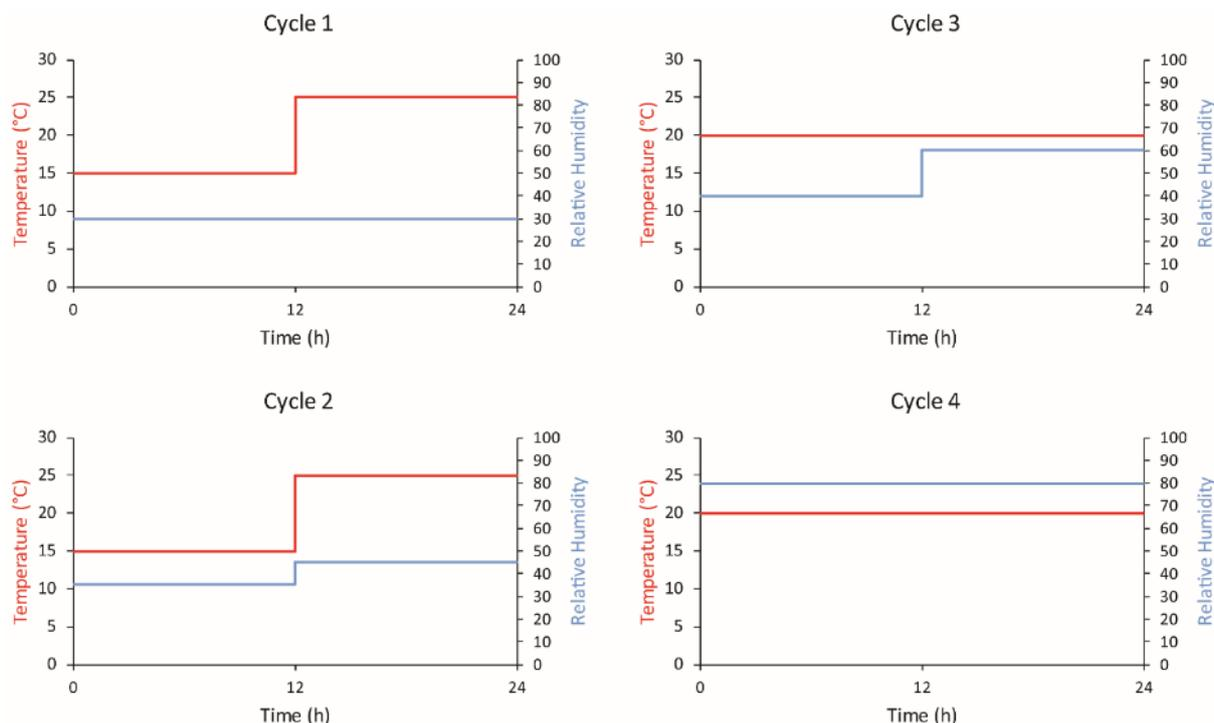
**Figure 6. Diagrams showing the temperature (°C) and humidity (%) parameters used for the four weathering cycles.**
