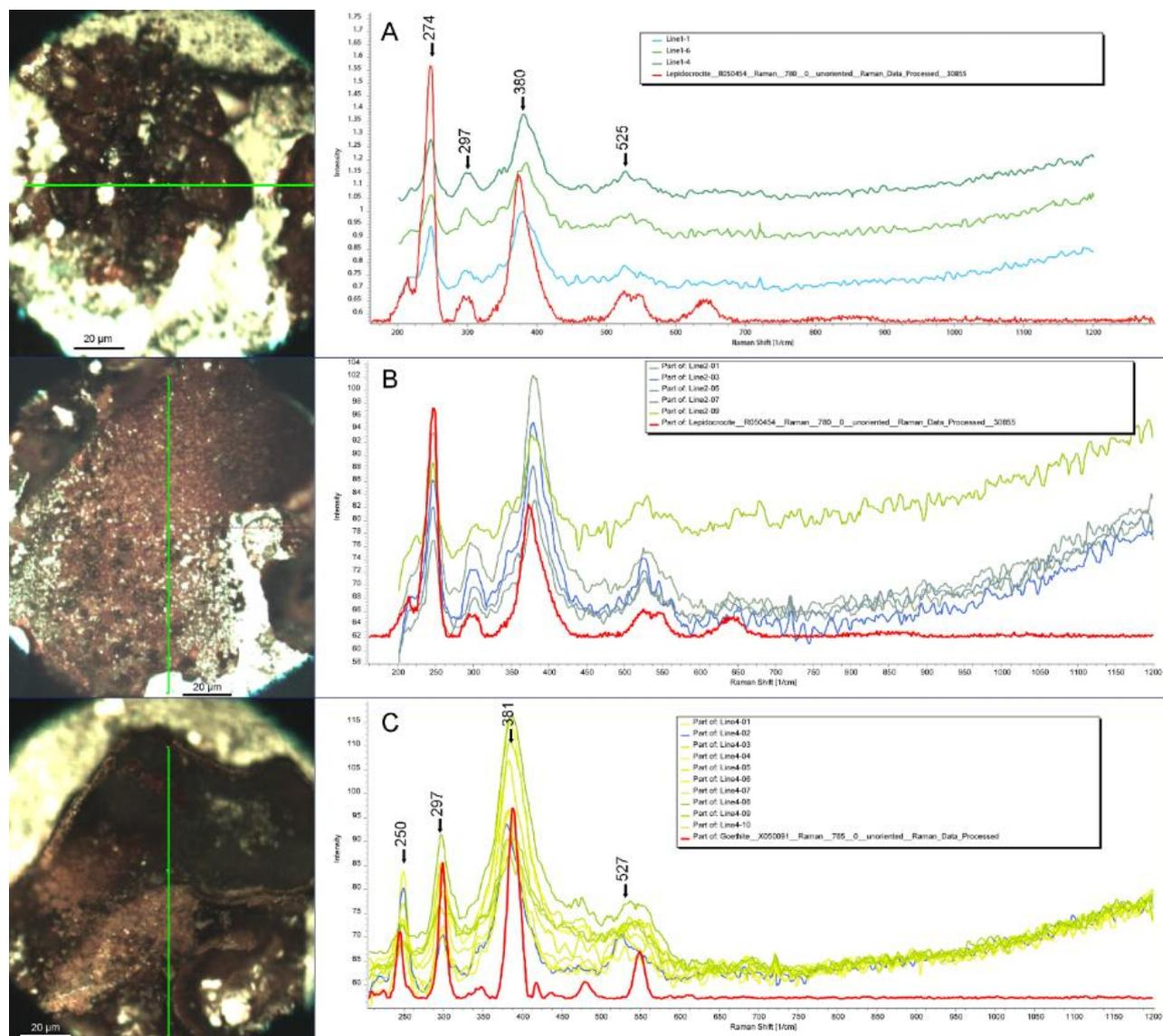
**Figure 21. Raman spectra of weathering products in MET-3. All line analyses (green lines on optical images). A and B) most weathering products show a match with the spectrum of lepidocrocite (red line; RRUFF ID: R050554). C) some weathering products show a match with the spectrum of lepidocrocite (red line; RRUFF ID: R050554). C) some weathering products show a match with goethite (red line; RRUFF ID: X050091).**
