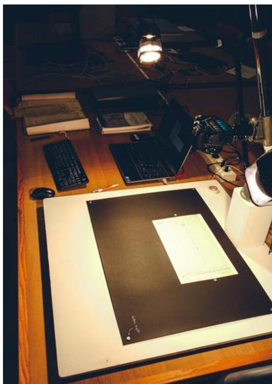
Figure 2: Digitization set-up including reproduction stand, lights, computer for direct image transfer and a background mask
