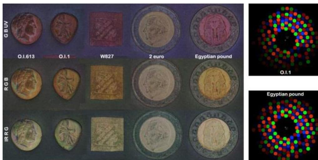
Figure 39: False colour representations and 2 examples of spectral reflectance responses on the collection of coins (MS PLD, © ESAT-VISICS, KU Leuven)
