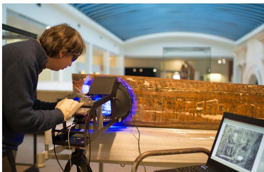
Figure 24: Imaging a decorated yellow coffin from the Egyptian collection of the RMAH: MS Microdome on tripod (© KMKG-MRAH)
