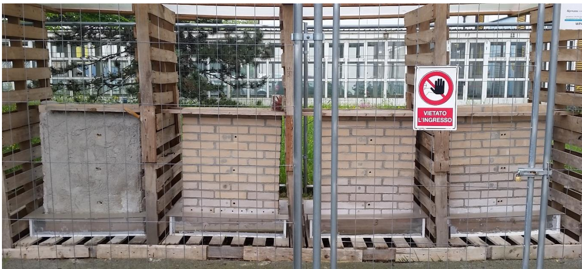
Figure 75: April 2016, 12 months after the treatment. The scale models seem to be dry (even the untreated scale model on the right). This effect arises from the fact that the weather is drier and warmer, thus causing the salts to dry out, as the relative humidity outside goes under the critical relative humidity of NaCl, around 75% RH.
