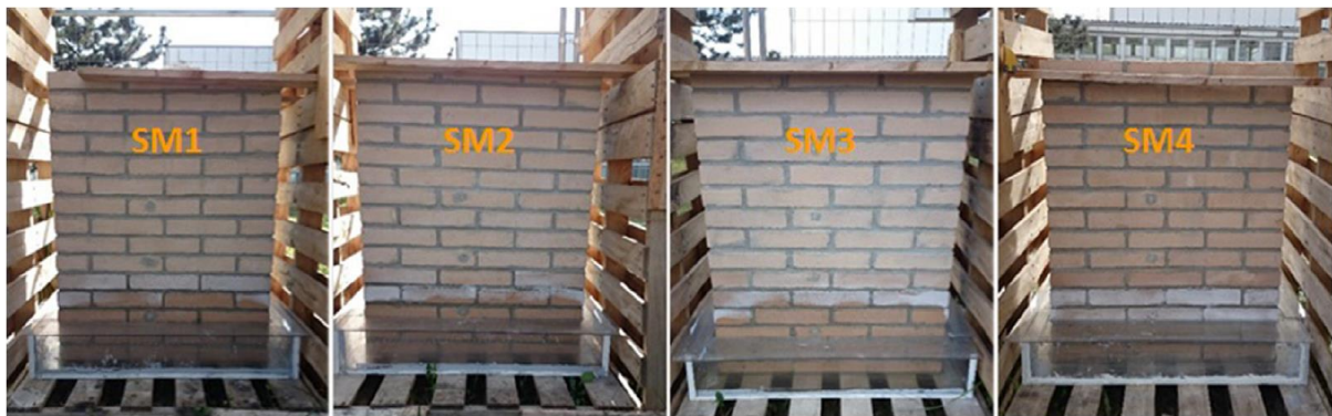
Figure 72: an overview of the 4 scale models, right before the treatments were applied. The humid zone, together with the expected salt efflorescences above the humid zone, are clearly visible. It is necessary to indicate that at this stage, no equilibrium is obtained: the rising damp has not yet reached its full height (usually in the order of 1 meter). But as the injection zone is already damp, at this stage the treatments can be carried out. It should be emphasized that at that very moment, the most salt-loaden zone (indicated by the efflorescences) is at a height around 20 cm above the water level. This is an important factor to fully understand the humidity distribution graphs (see below).
