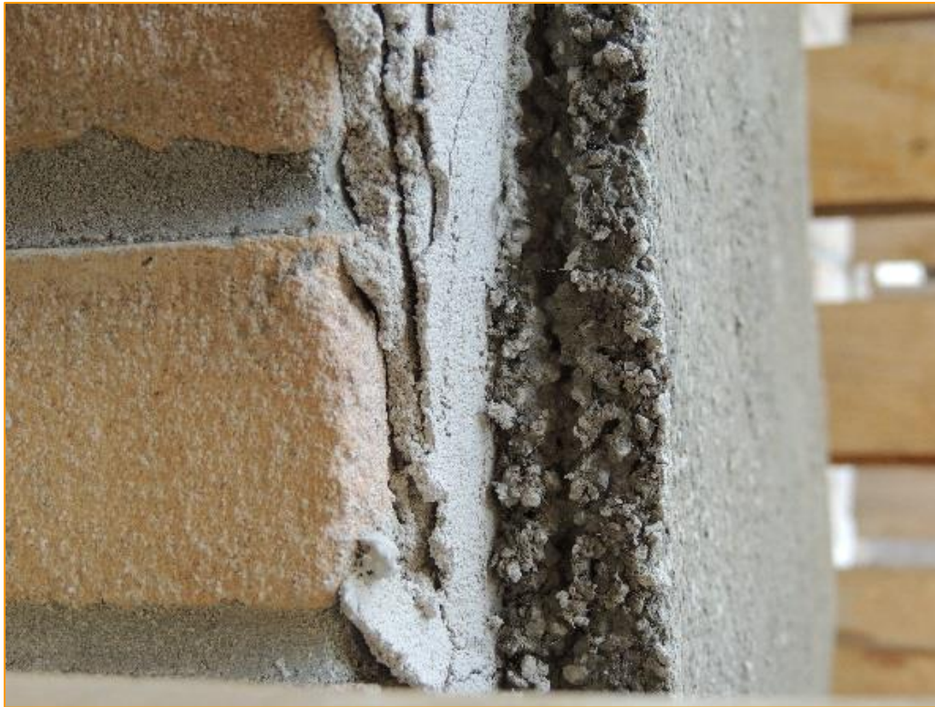
Figure 73: detail, showing the two layers of dehumidifying plaster on Scale model 4. One can clearly see the different thicknesses of the two layers, and their difference in nature.
