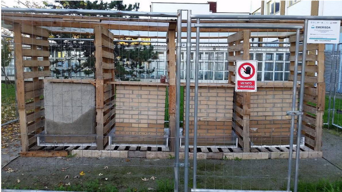
Figure 74: November 2015, 7 months after the treatment. One can clearly see lots of humidity in the scale models. At least part of this humidity is hygroscopic humidity, caused by hygroscopic water uptake by the salts in humid cold weather.
