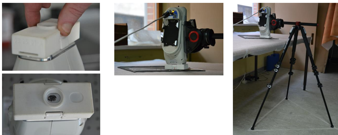
Figure 42: Illustration of the so-called 'XRF nose' which is a component that is mounted to the measuring head of the p-XRF device ensuring the implementation of a constant distance
