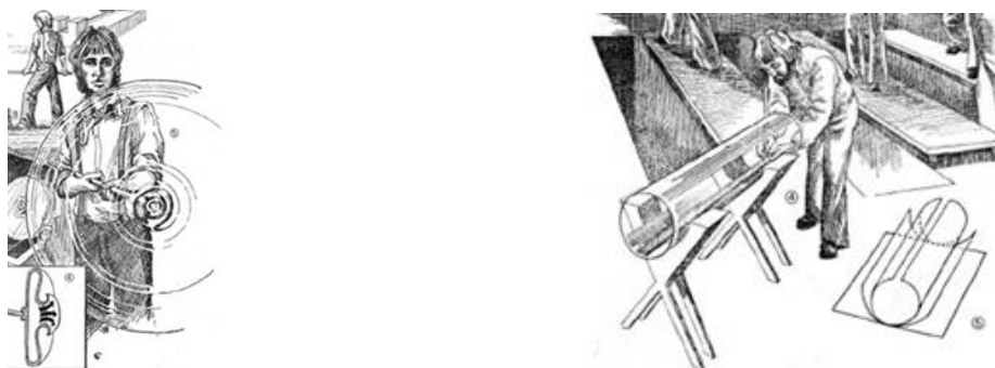
Figure 3: Glass fabrication with the crown (left) and the cylinder (right) techniques. Pictures are taken from (Dungworth, 2011)
