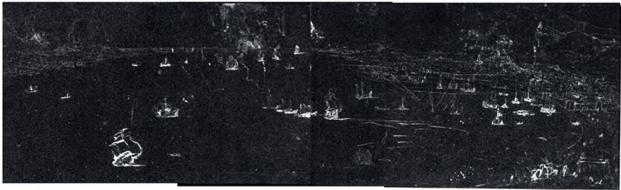
Fig. 27.7 Recto of View of the Strait of Messina (fig. 27.1). MA-XRF image. Fe-K \alpha distribution map, visualizing the iron component in the iron gall ink
