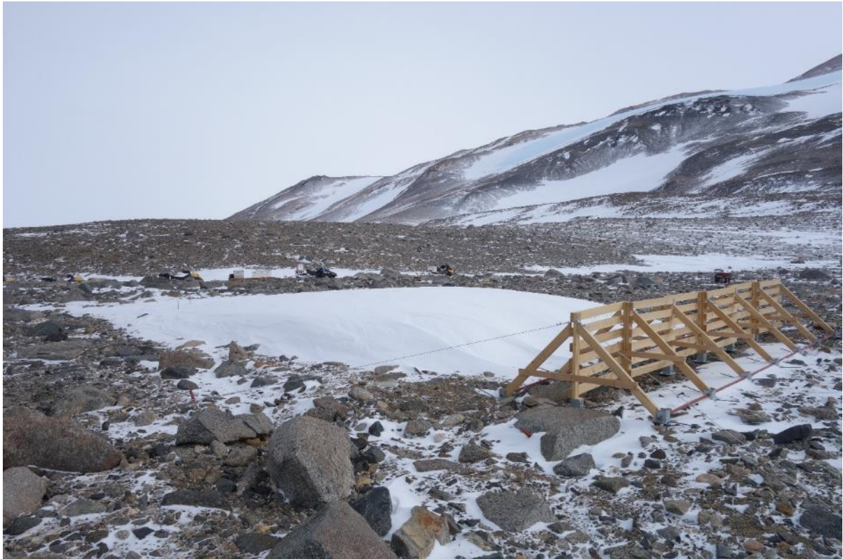
Fig. 4.2.5: One of the two snow fences in the Dry Valleys region. Turbulence caused by the fences allows snow to collect downwind of the snow fence.
