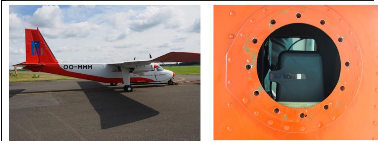
Figure 17. The Mumm BN-2 in Antwerp Airport and SWING integration on-board (28 July 2016)
