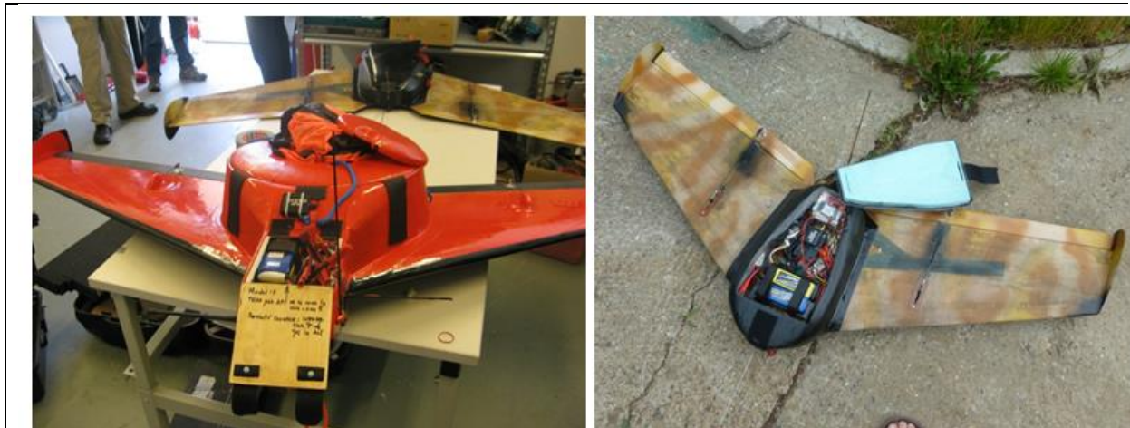
Figure 26. (left) The large wing in the front, the small wing in the back. The central cylindrical box in the large wing contains the aircore and landing parachute; the nose contains the GPS, all electronics and radiosystem. (right) the small wing with GPS, all electronics and radiosystem in the central position. This wing is for test purposes only; there is no space provided for the payload.
