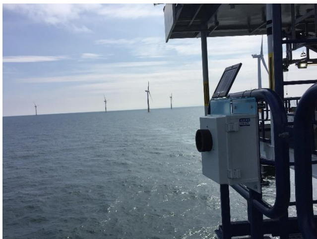
Figure 1. Bat detector installed in a wind farm at sea.
