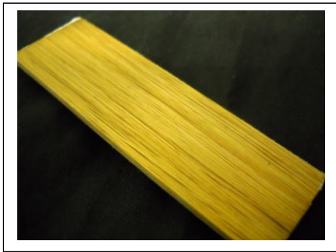
Figure 4: Bamboo fibre composite plate
