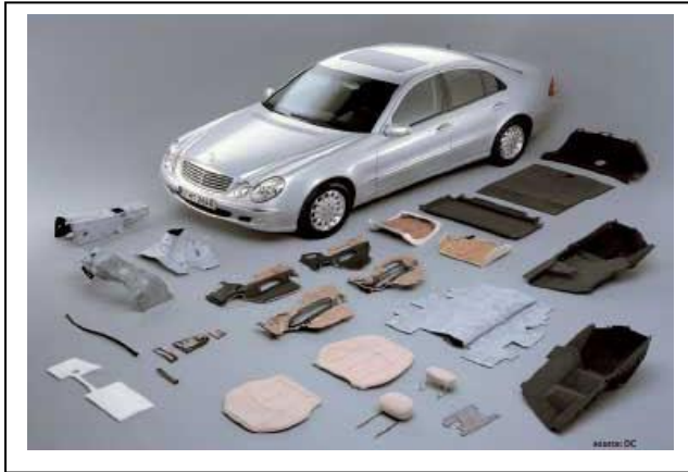
Figure 6. Applications of natural fibre components in automotive parts. Picture source: http://www.ircomas.org
