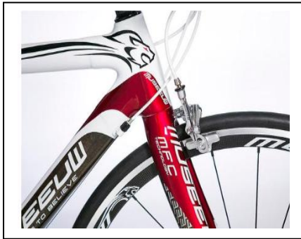
Figure 7. Recent application of natural fibres in bicycle frames for increased material damping. Picture source: http://www.lineo.eu/
