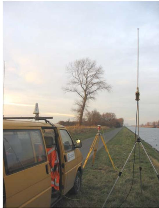
**Picture 2b:** Survey position GPS and radio antennas.
