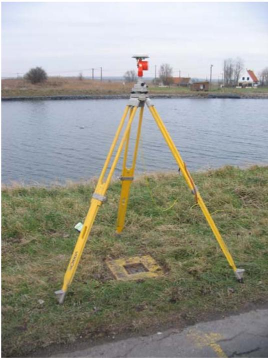
**Picture 3a:** Position of the GPS antenna on top of the geodetic benchmark.
