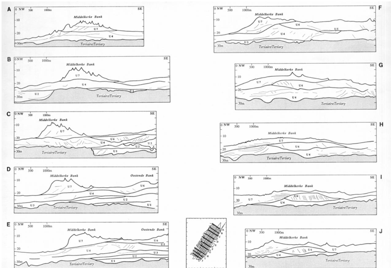
Figure 17: Seismic units composing the internal structure of the Middelkerke Bank (selected interpreted seismic sections from A to J) (Berné et al., 1994).
