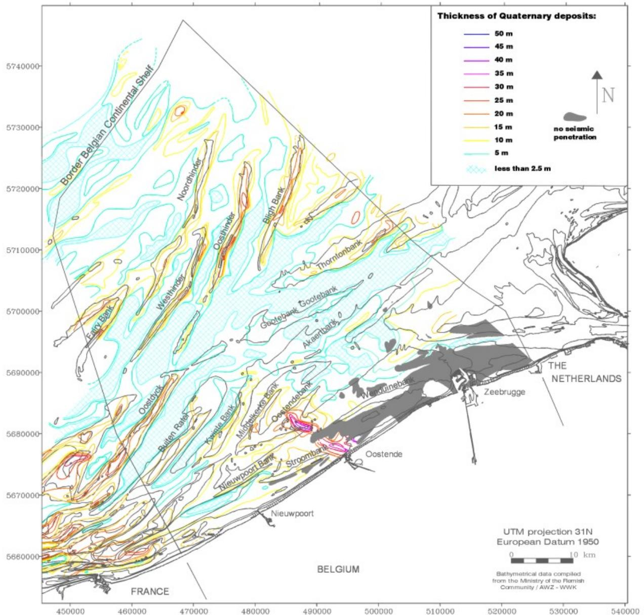
Figure 23: Thickness of Quaternary sediments (after Liu, 1990).
