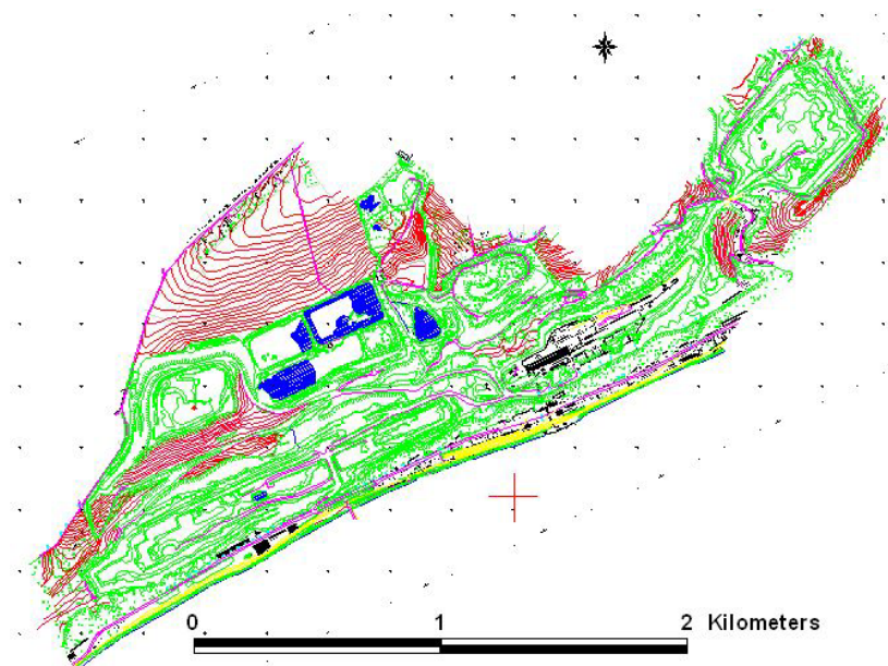
Figure 30 Site of Amay with measured elevation data and the height contour lines
