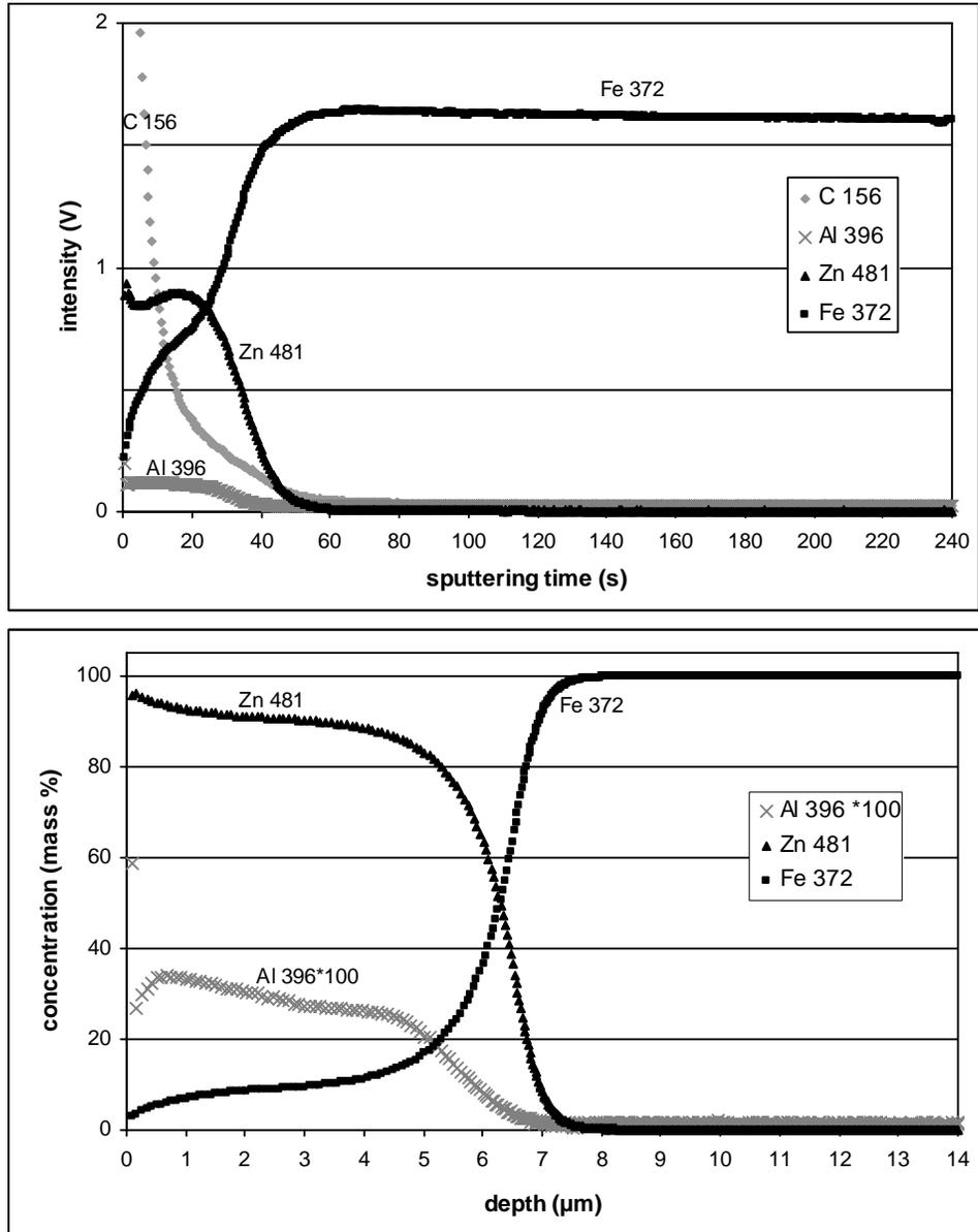
Figure 19. Qualitative depth profile (top) and compositional depth profile (bottom) of sample “galvannealed”. The mass% values for aluminium were multiplied by 100 for visibility.
