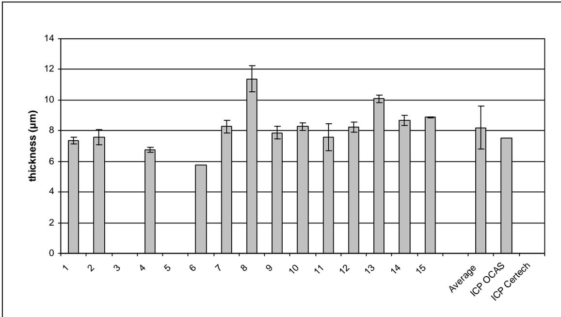
Figure 21. Interlaboratory comparison. Results for thickness of GI, with standard deviation.
