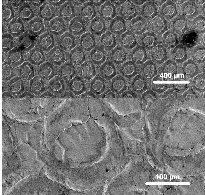
Figure 2. Morphology of the surface of coating GI as observed in SEM. Overview and detail.
