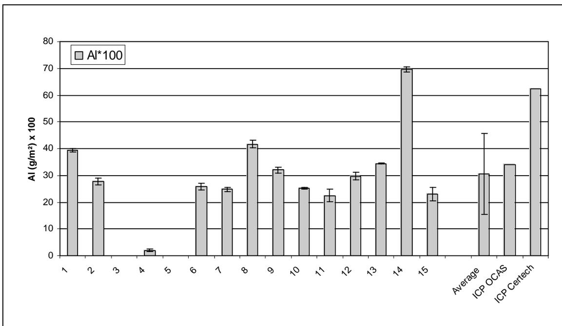
Figure 23. Interlaboratory comparison. Results for aluminium in GI, with standard deviation.
