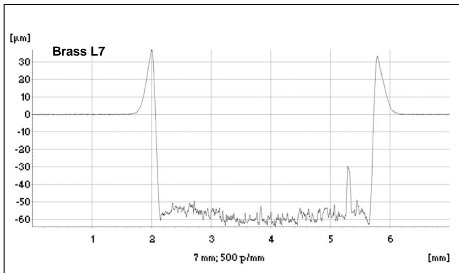
Figure 7. Example of a crater profile in the calibration sample brass L7. Crater depth is close to 60  $\mu\text{m}$ . Sputtering time was 10 min.
