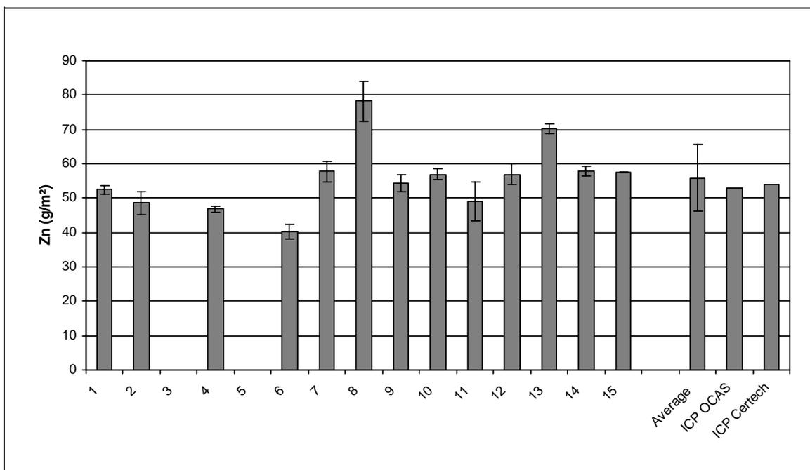
Figure 22. Interlaboratory comparison. Results for total zinc in GI, with standard deviation.
