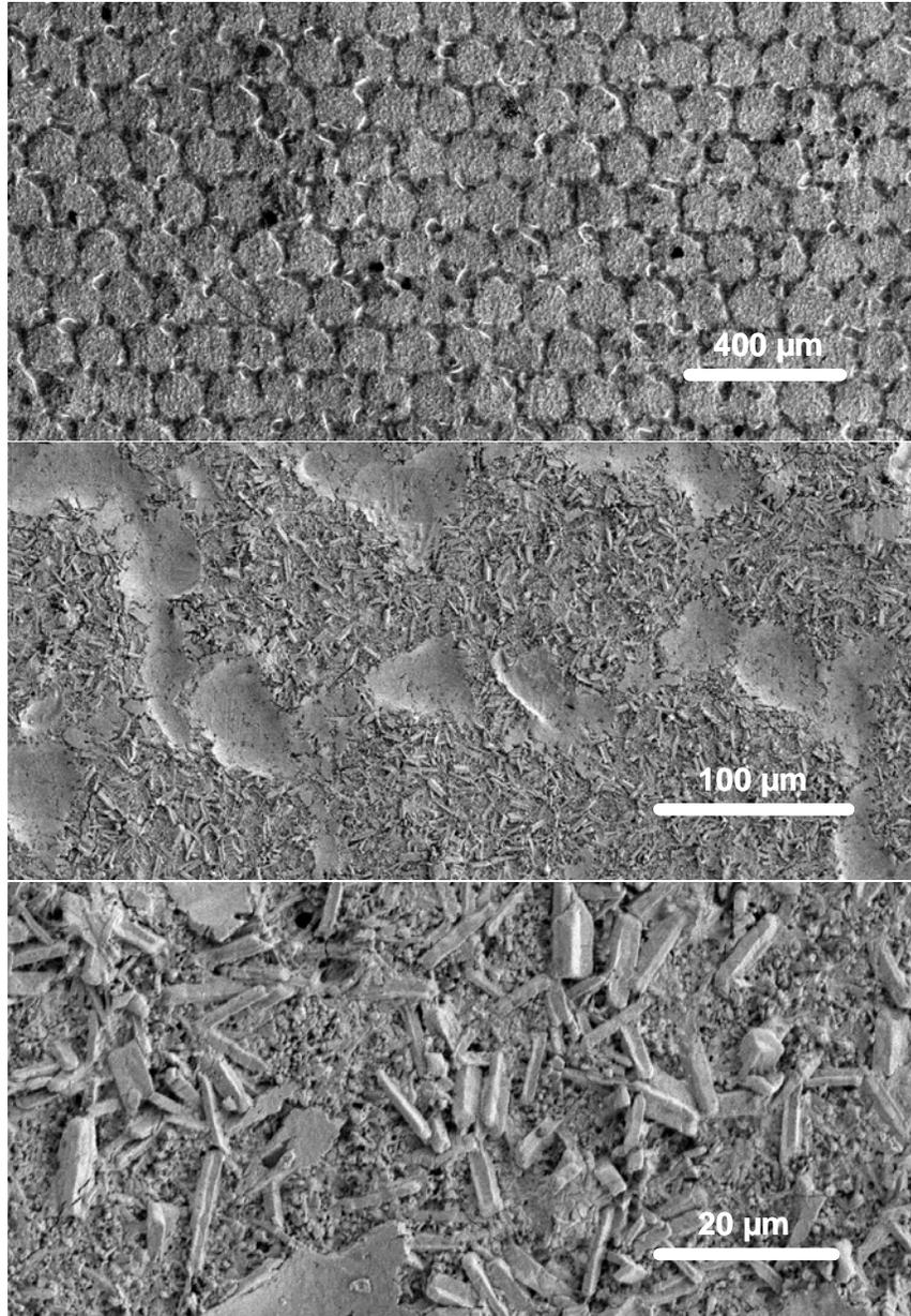
Figure 3. Morphology of the surface of coating GA as observed in SEM. Overview and details.
