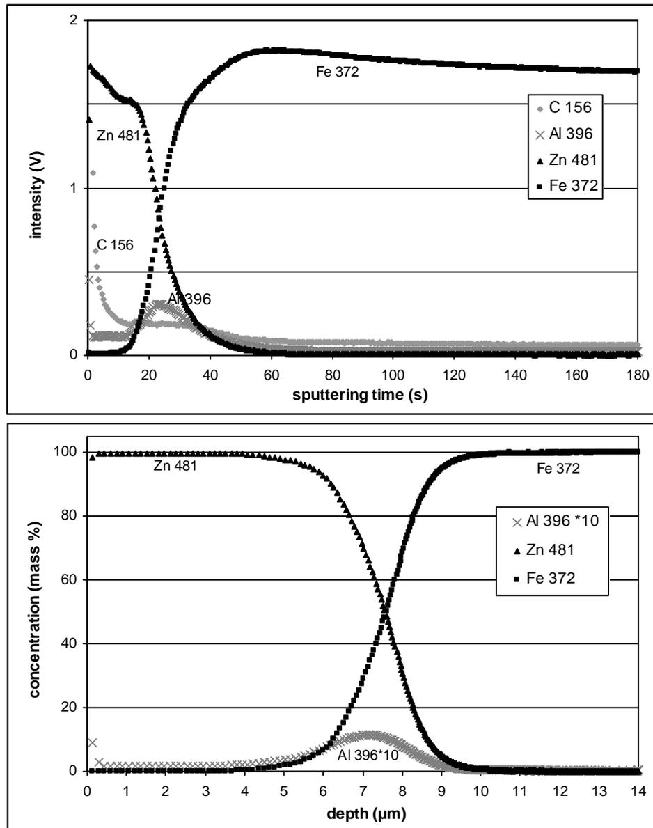
Figure 15. Qualitative depth profile (top) and corresponding compositional depth profile (bottom) of the hot dip galvanized sample GI. The mass% values for aluminium were multiplied by 10 for visibility.
