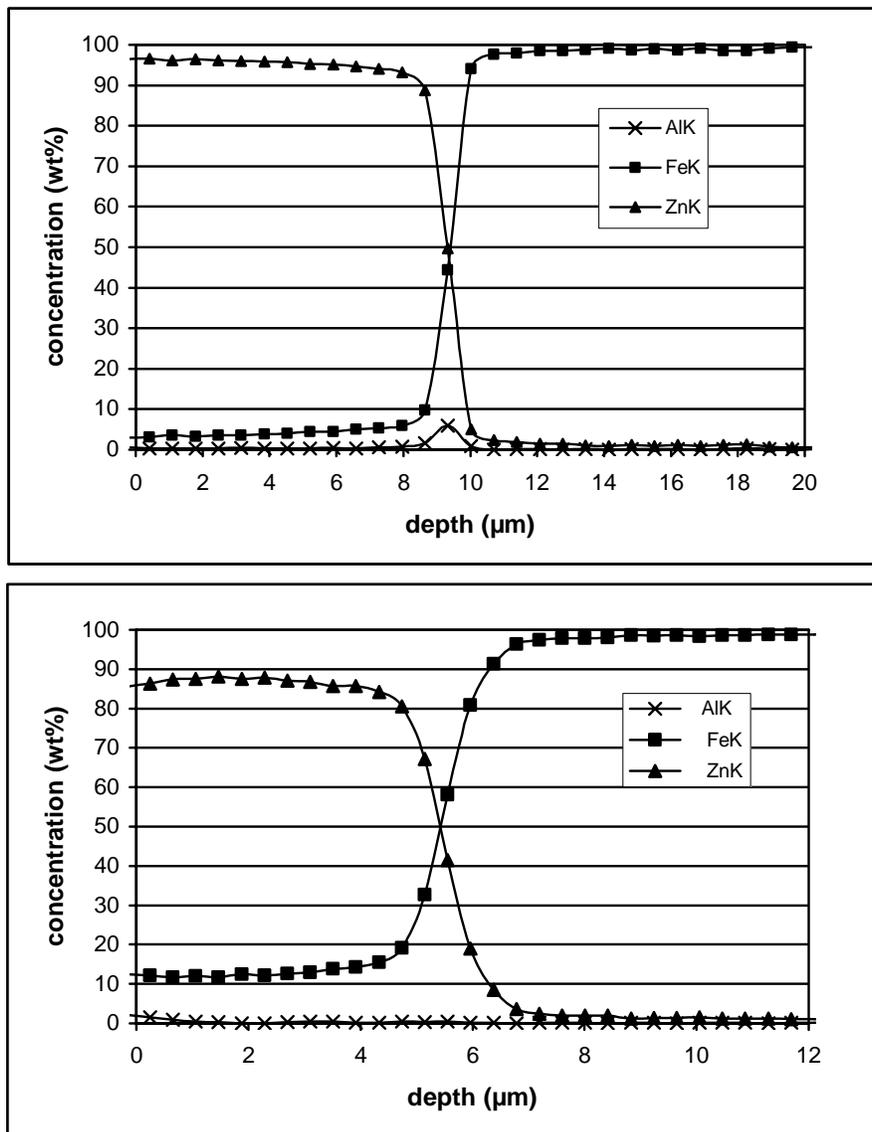
Figure 6. EDXA line scans over the cross sections of GI (top) and GA (bottom).
