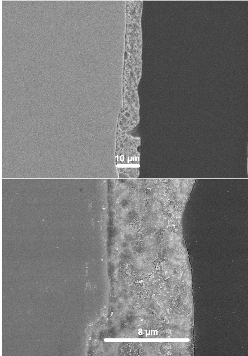
Figure 4. Cross-section of the coating GI on its substrate, as observed in SEM. Overview and detail.
