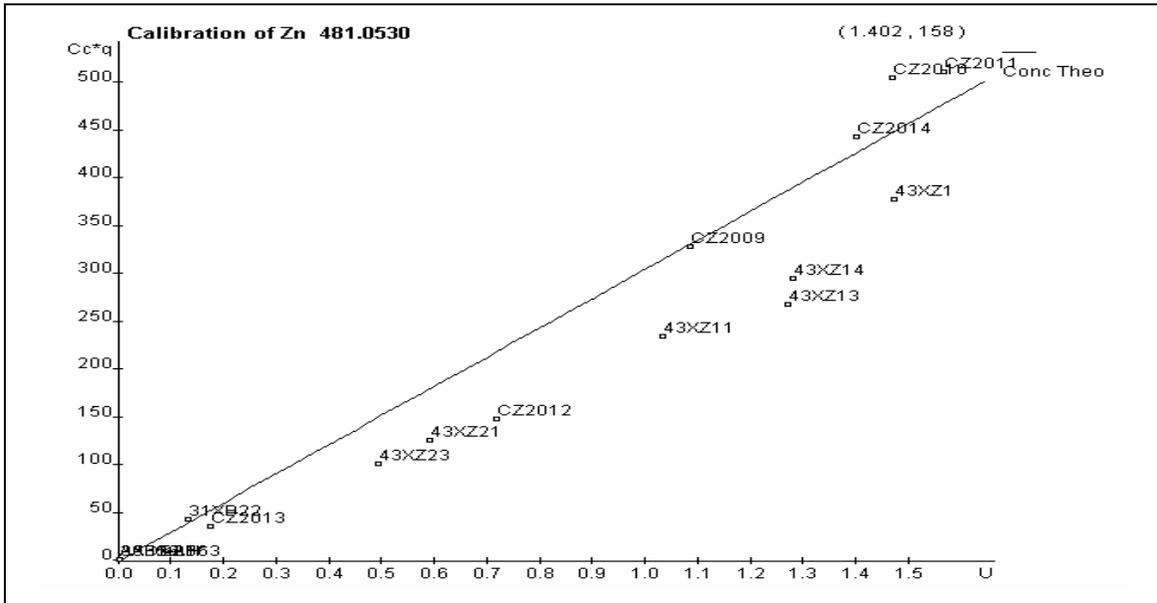
Figure 9. Calibration graph for zinc, excluding most of the brass samples, but including the zinc-rich CMI samples. Note the apparent separation between CMI and MBH zinc-alloys. The weight of the MBH samples was deliberately decreased to include some of the more zinc-rich CMI samples.
