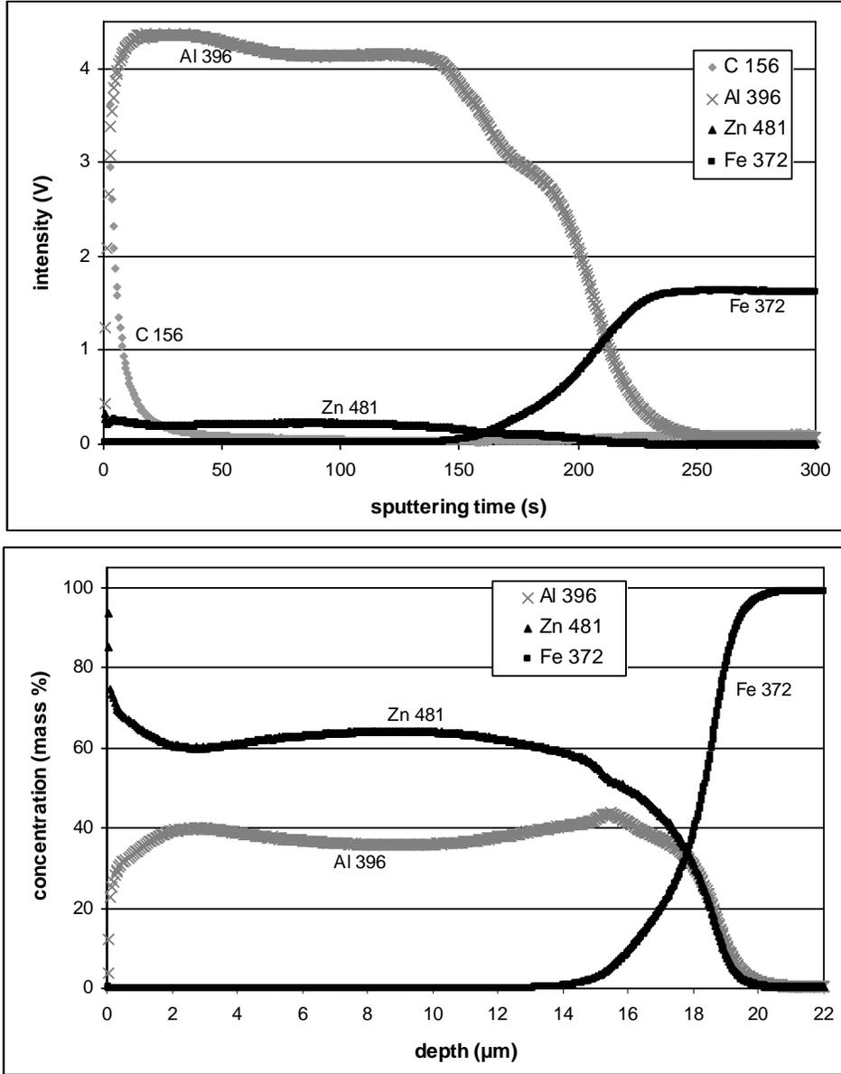
Figure 20. Qualitative depth profile (top) and compositional depth profile (bottom) of aluzinc test sample “aluzn”.
