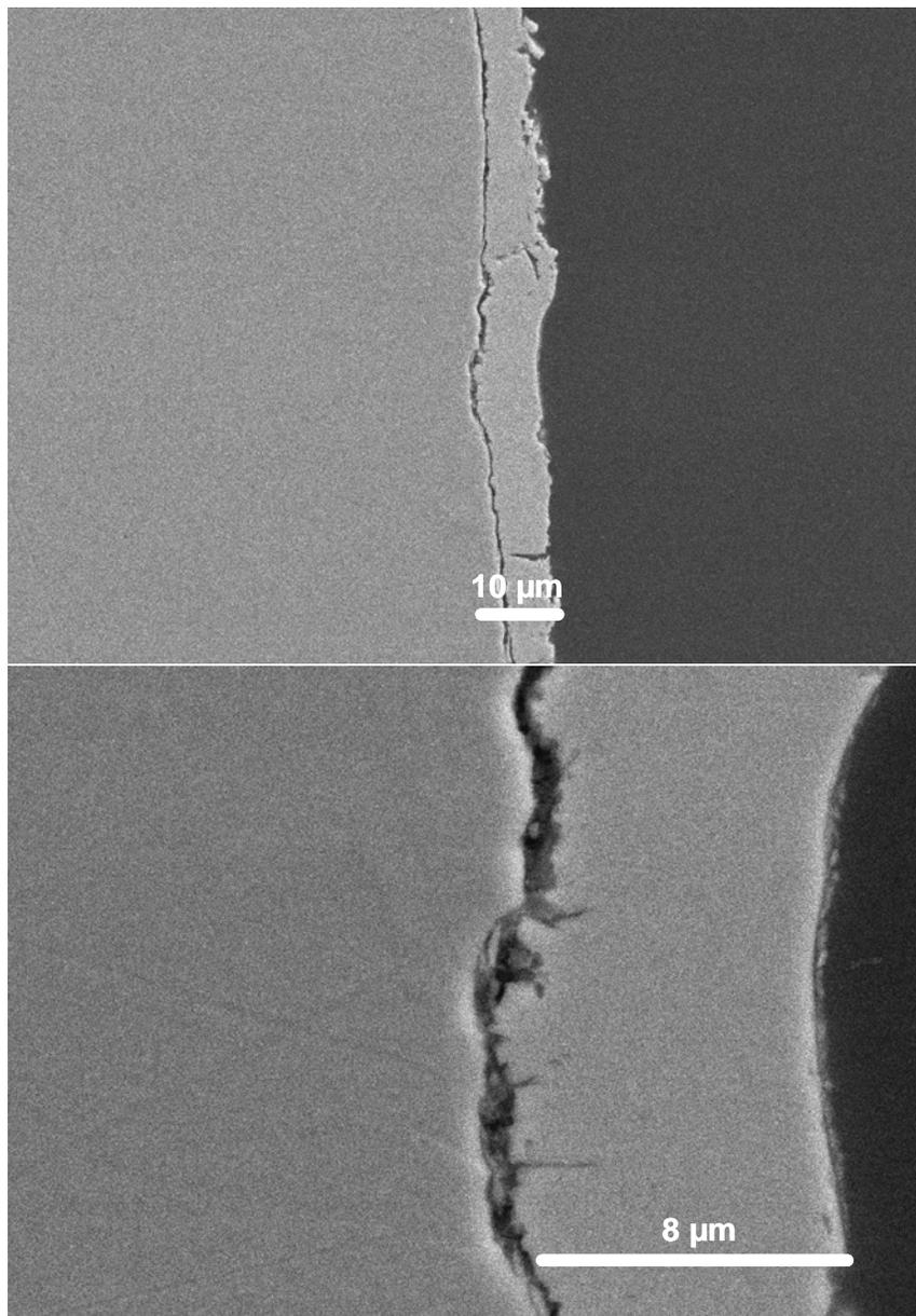
Figure 5. Cross-section of the coating GA on its substrate, as observed in SEM. Overview and detail.
