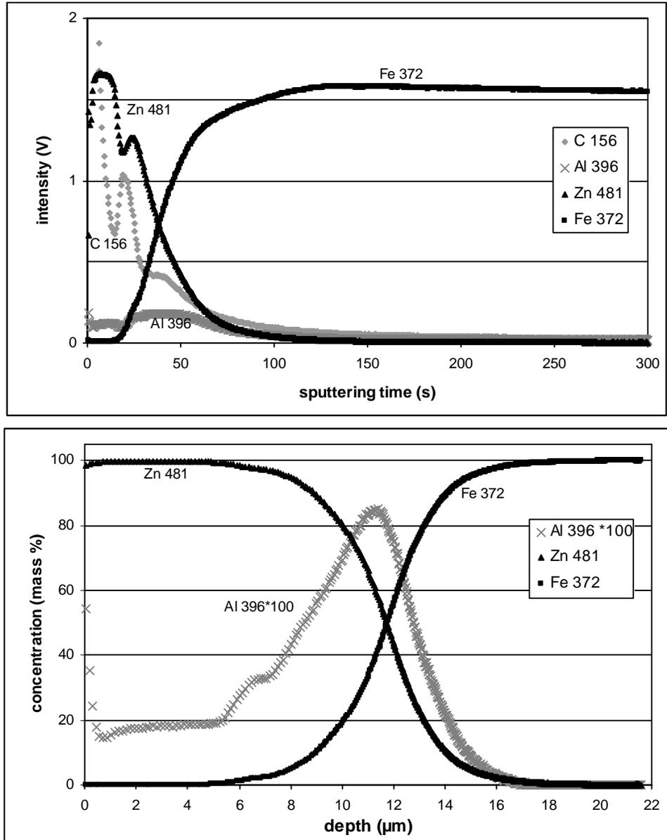
Figure 17. Qualitative depth profile (top) and compositional depth profile (bottom) of galvanized test sample 9025M. The mass% values for aluminium were multiplied by 100 for visibility.
