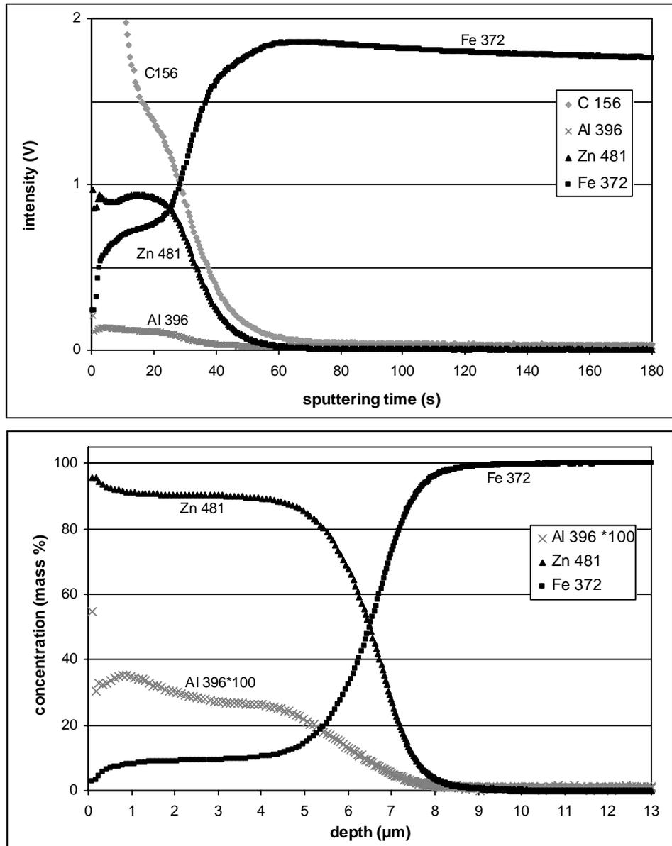
Figure 16. Qualitative depth profile (top) and corresponding compositional depth profile (bottom) of the galvanneated test sample GA. The mass% values for aluminium were multiplied by 100 for visibility.
