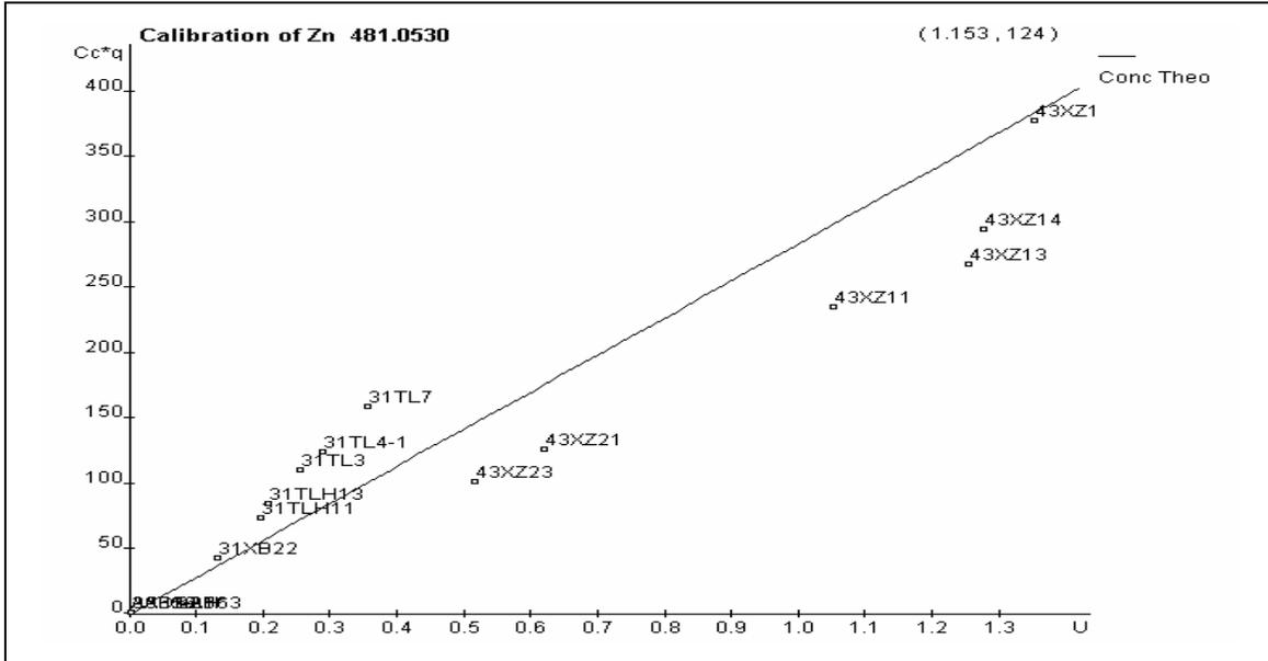
Figure 8. Calibration graph for zinc, including the brass samples. The separation between brass and zinc-aluminium matrices can clearly be distinguished (§2.6.4).
