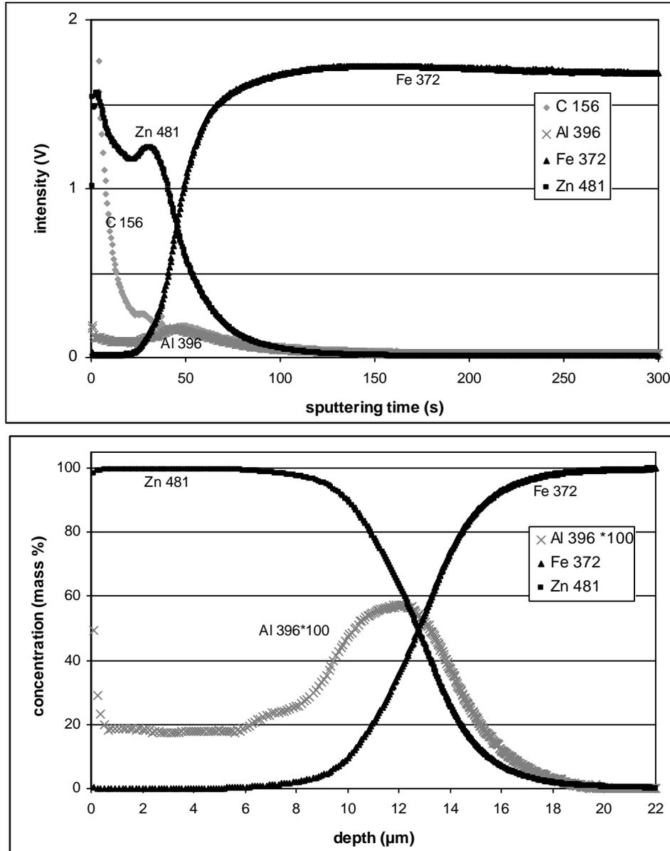
Figure 18. Qualitative depth profile (top) and compositional depth profile (bottom) of galvanized test sample 9100. The mass% values for aluminium were multiplied by 100 for visibility.
