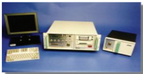
>> Figure 81: Monitor (left), control unit (middle) and optical sensor head (right) of the CASI-2 sensor (ITRES Research Limited, Canada).
