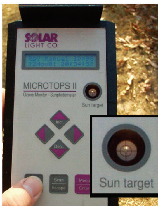
>> Figure 87: MICROTOPS II sun photometer and the sun target.
