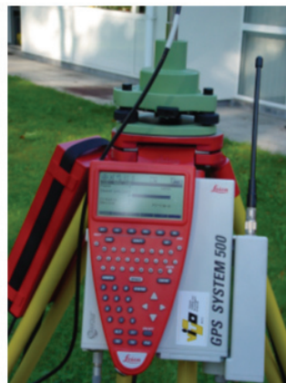
>> Figure 34: Leica SR530 base station GPS.
