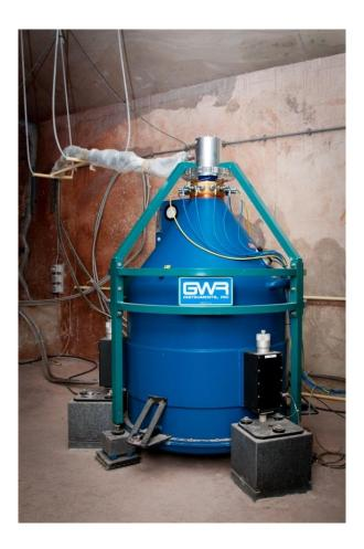
The superconducting gravimeter is installed at the end of a 140 m-long gallery, excavated under the "Hertogenwald" forest, between the reservoirs of Eupen and La Gileppe.
