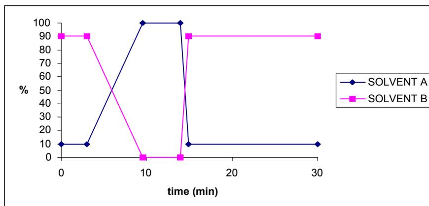
Figure 4. LC-MS/MS gradient used for the elution of OTA
