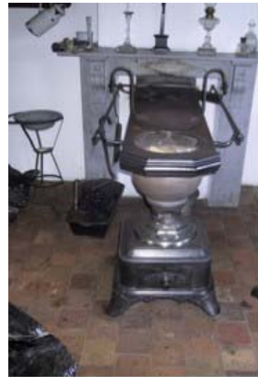
Figure 59 : Picture of a "Leuvense stoof" used for emission measurements in Bokrijk
