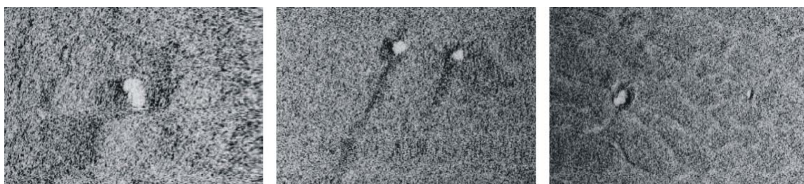
Fig. 12: Side-scan sonar images of obstacles. The block are 2-3 m in diameter.
