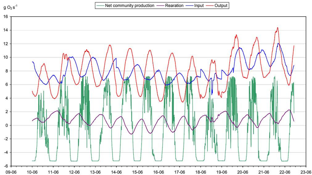
Figure 63: A comparison between reactive fluxes in the river reach (net production, reaeration) and transport fluxes at the upstream and downstream boundaries. Results are given for run 3 (9 June – 23 June 2004).
