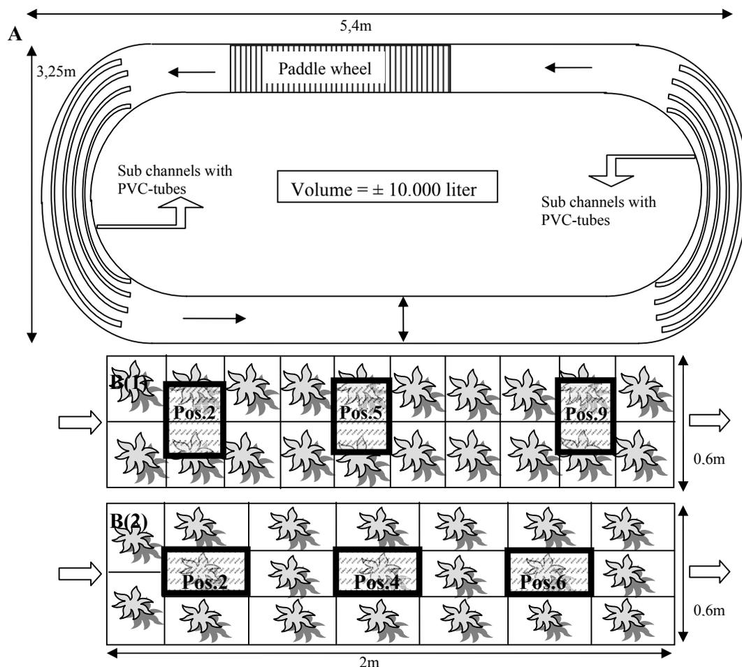
Figure 33: (A) schematic presentation of the flume (top view) and (B) schematic presentation of the arrangement of 20 pots with macrophytes in the test section for (1) *Callitriche platycarpa* and *Potamogeton natans* and for (2) *Sparganium erectum*. \* = macrophytes in each pot. The black rectangles with biomass were selected to analyse  $^{15}\text{N}$  in the biomass standing in the different locations in a patch.
