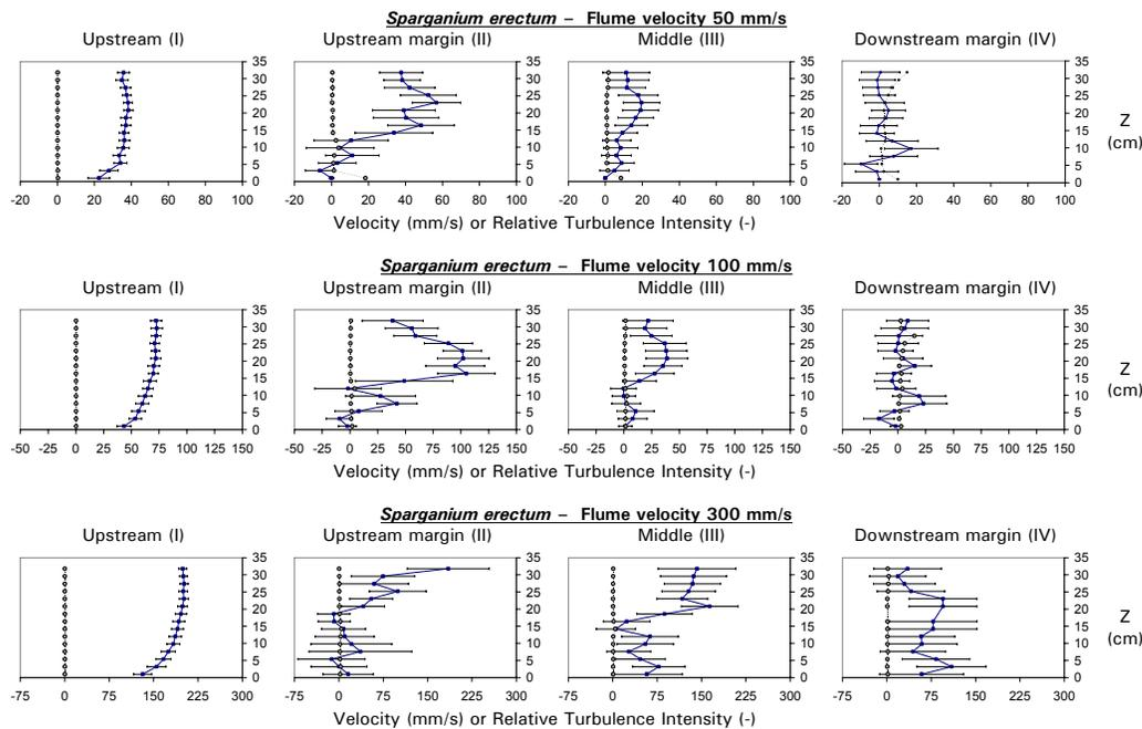
Figure 40-42: Real velocity ( $\text{mm s}^{-1}$ ) and Turbulence Intensity (-) patterns for *Sparganium erectum* at three enforced velocities (50, 100 and  $300 \text{ mm s}^{-1}$ ) upstream the patch (I), in the upstream margin of the patch (II), in the middle of the patch (III) and at the downstream margin of the patch (IV).
