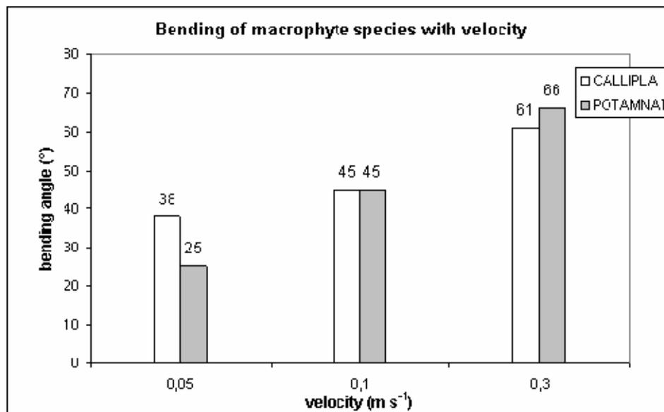
Figure 43: Bending angle of *Callitriche platycarpa* and *Potamogeton natans* with three current velocities. Bending angles of *Sparganium erectum* are not plotted on the graph because no bending could be observed.
