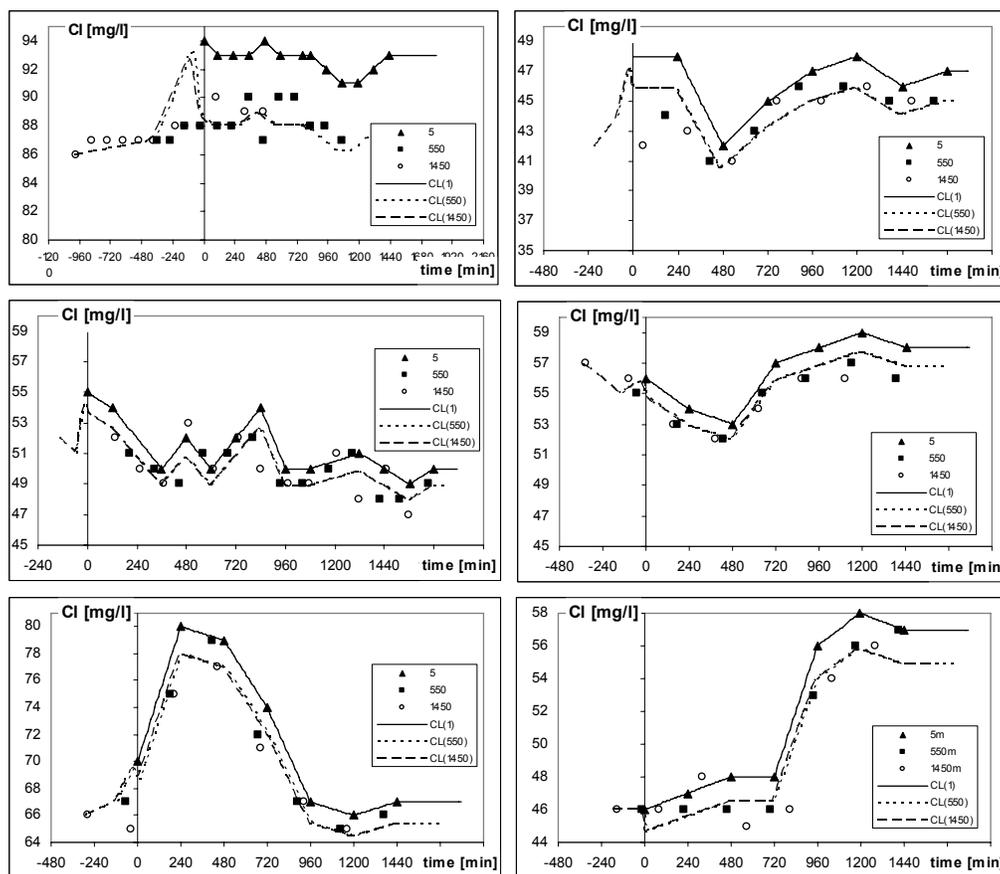
Figure 21: Tracer chloride values [ $\text{mg l}^{-1}$ ] at the upstream weir (▲), in the middle (■) and at the downstream weir (○) for the six campaigns plotted against relative time [min]. Accordingly, the behaviour of one water package is shown. Dotted lines represent chloride values obtained by modelling the dilution originating from the Sloopbeek only in the middle (..... CL(550)) and at the downstream weir (— — CL(1450)).
