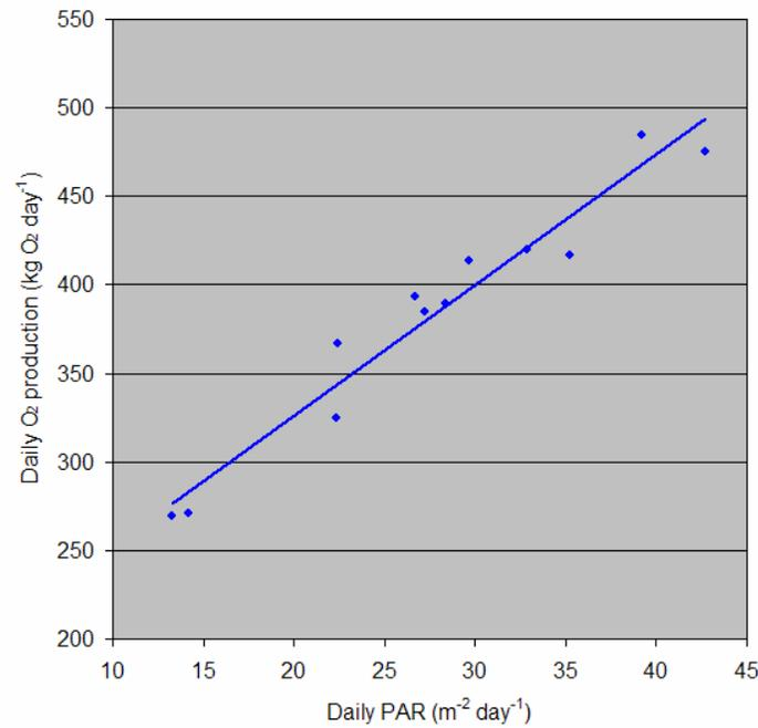
Figure 65: Daily O<sub>2</sub> production as a function of daily irradiance, for run model #3. (O<sub>2</sub> prod = 0.0167 PAR,  $r^2 = 0.95$ )
