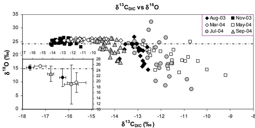
Figure 28. Seasonal variation in the  $\delta^{13}\text{C}_{\text{DIC}}$  and  $\delta^{18}\text{O}_{\text{DO}}$  composition in the Aa River 2003-2004. The insert shows the mean ( $\pm$  SD) of all months. The dashed line represents the  $\delta^{18}\text{O}_{\text{DO}}$  value for a situation where  $\text{DO}$  is in equilibrium with air  $\text{O}_2$  (24.2‰).
