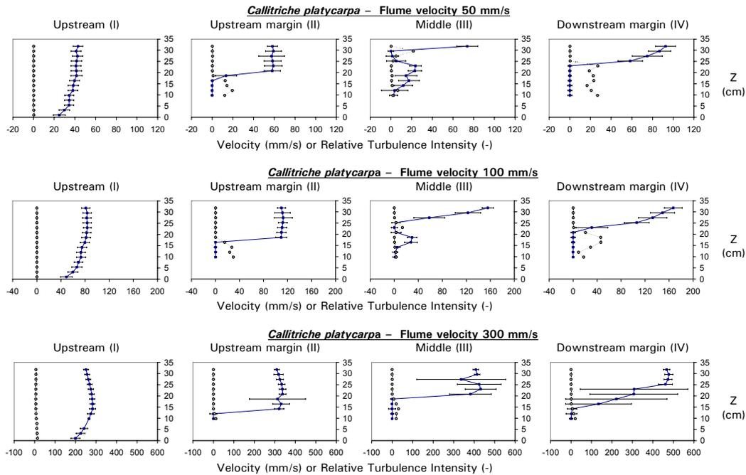
Figure 34-36 Real velocity ( $\text{mm s}^{-1}$ ) and Turbulence Intensity (-) patterns for *Callitriche platycarpa* at three enforced velocities (50, 100 and  $300 \text{ mm s}^{-1}$ ) upstream the patch (I), in the upstream margin of the patch (II), in the middle of the patch (III) and at the downstream margin of the patch (IV).
