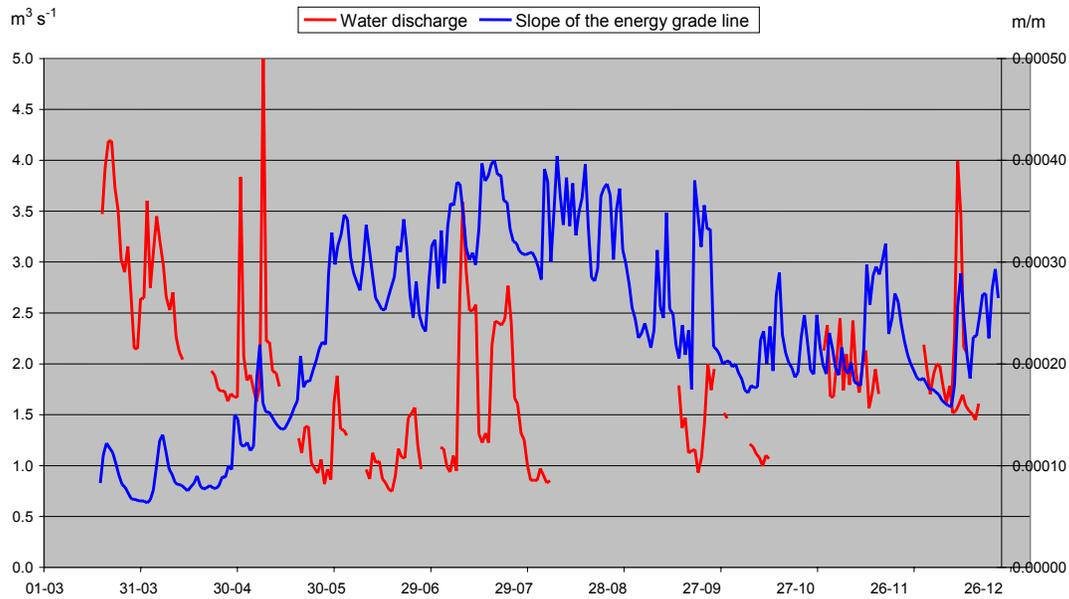
Figure 54: Seasonal evolution of the water discharge and of the slope of the energy grade line (2004)
