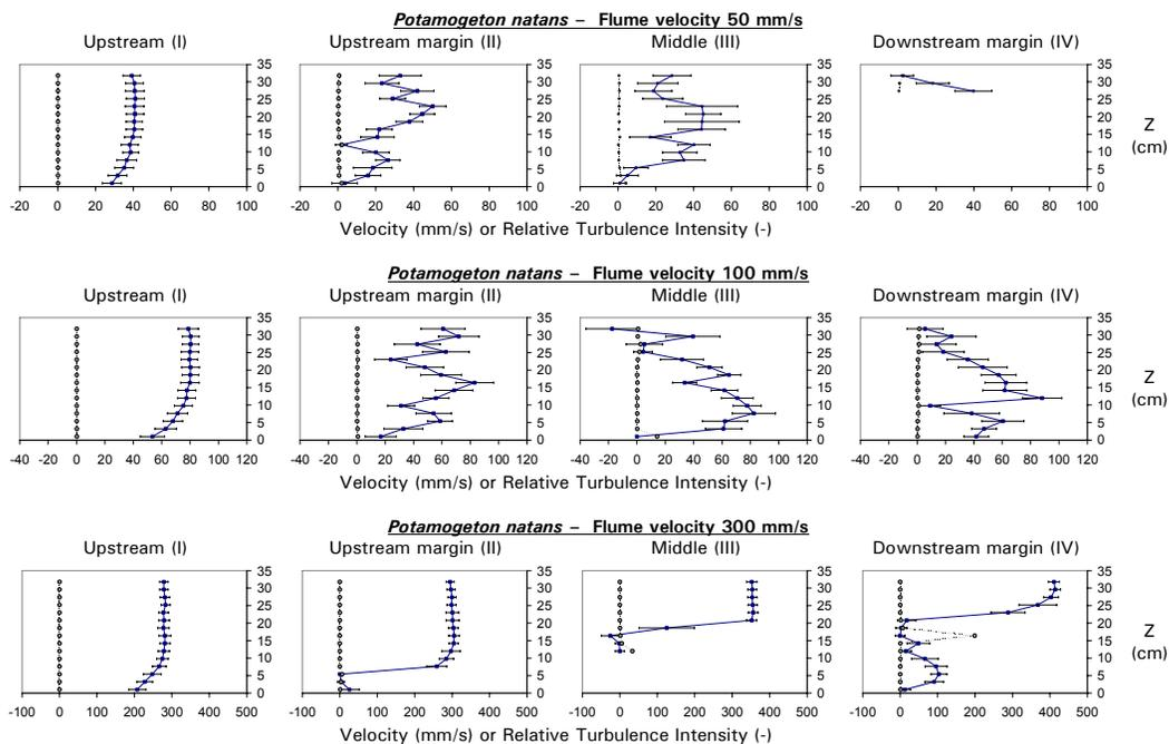
Figure 37-39: Real velocity ( $\text{mm s}^{-1}$ ) and Turbulence Intensity (-) patterns for *Potamogeton natans* at three enforced velocities (50, 100 and  $300 \text{ mm s}^{-1}$ ) upstream the patch (I), in the upstream margin of the patch (II), in the middle of the patch (III) and at the downstream margin of the patch (IV).
