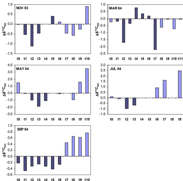
Figure 31: Seasonal variation in the diurnal change in δ<sup>13</sup>C<sub>DIC</sub> ( $\Delta\delta^{13}\text{C}_{\text{DIC}} = \delta^{13}\text{C}_{\text{DIC}(\text{gate } 4)} - \delta^{13}\text{C}_{\text{DIC}(\text{gate } 3)}$ ) between gate 3 and gate 4 in the Aa River 2003-2004. The shaded bars denote samples taken between sunset and sunrise. Note that the amplitude of the changes are largest during May and July 2004.
