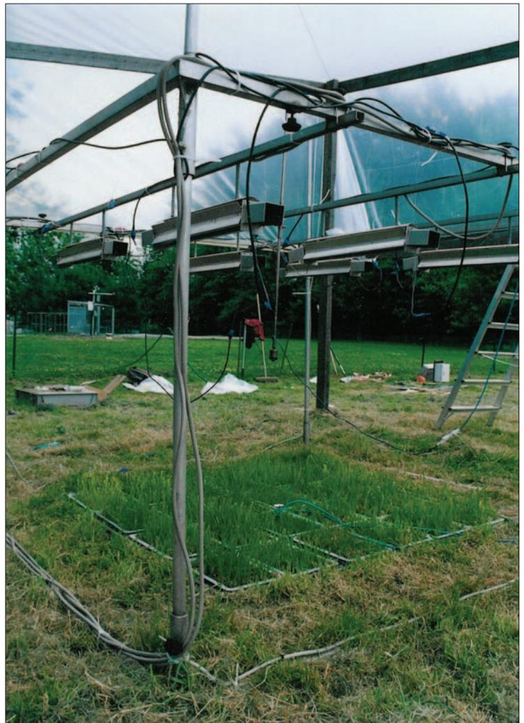
Figure 4.1- Simulation of natural heat waves with suspended infrared heaters (Free Air Temperature Increase technique) at UA. Below the heaters are containers with artificially composed grassland communities with different numbers of plant species, to verify whether loss of plant diversity affects sensitivity to extreme events. (I. Nijs, UA-PLECO).
