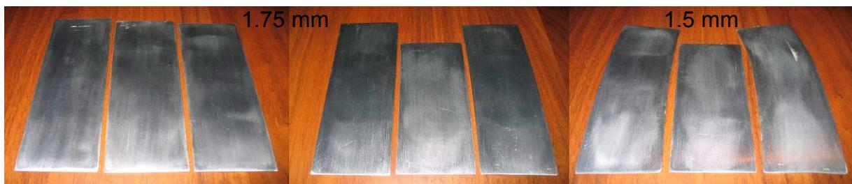
**Figure A.4.3: Strips after 6 passes of I-ECAP and machining with sand paper**
