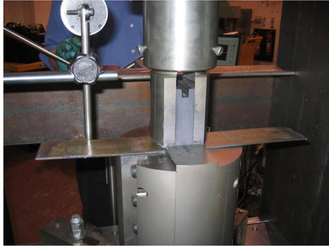
**Figure 2.7: Tool design for I-ECAP of sheets**
