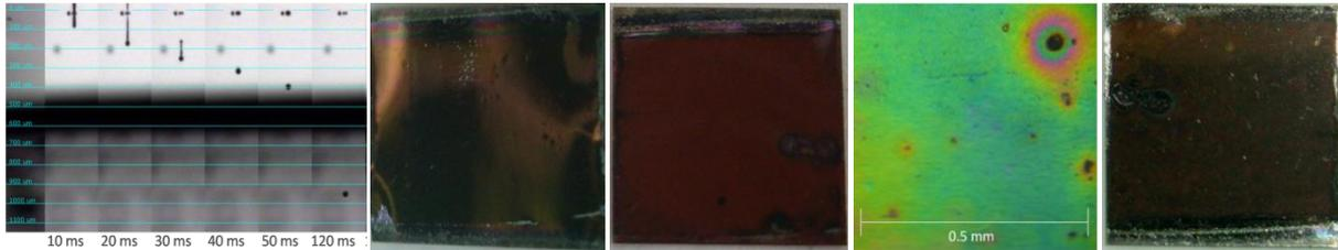
**Fig. 2.16: Droplet formation, coated substrate from liquid to 200°C (+ optical microscopy) and after 400°C**
