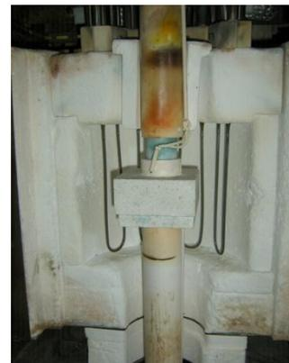
**Fig. 3.5: Uniaxial hot pressing setup**
