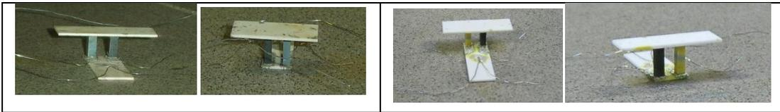
**Fig. 3.17: Module n°1 before (left pictures) and after annealing (right pictures)**
