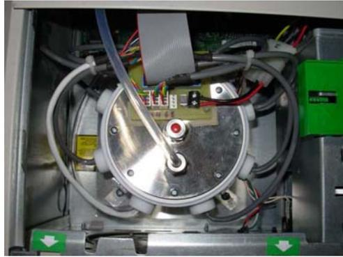
Figure 43 : E-nose sensor chamber
