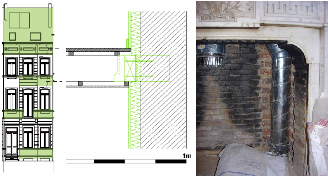
Figure 12: Insulation planning behind a protected façade and integration of mechanical ventilation in existing neoclassical chimney infrastructure (project avenue Rubens, Brussels demonstration programme; source: C. Jadoul, IEA workshop, see also [IBGE_09])
