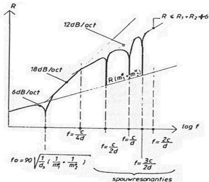
**Figure 21: Sound insulation of double walls: classical infinite wall theory (source: (Vermeir, 1999))**
