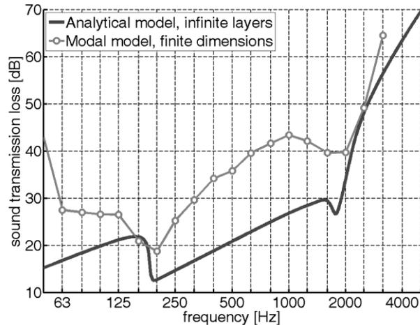
**Figure 22: Sound transmission loss of double glazing: influence of finite dimensions**
