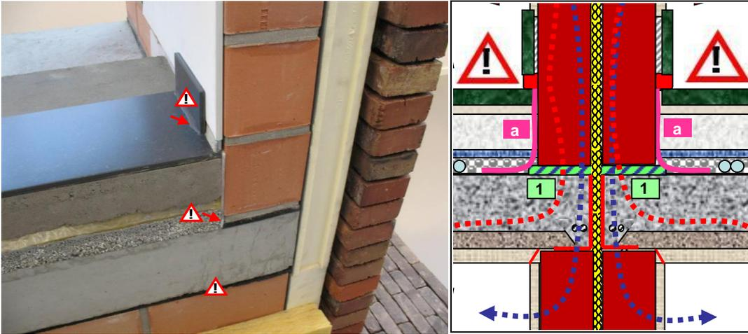
**Figure 45: IMPORTANT:** where resilient layers are employed (with middleweight construction shown in black in the left-hand figure, shaded green in the right-hand figure), the edge contact strips must at least reach the supporting floor and should preferably be folded onto it (see right-hand figure, point “a”)
