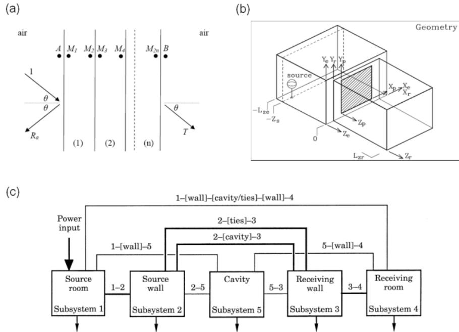
**Figure 20: Sound transmission loss models (a) Analytical models (b) Deterministic models (c) Statistical models**
