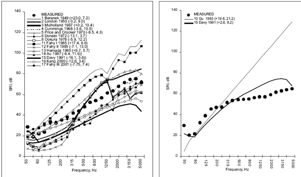
**Figure 23: Comparison of existing models with experiment: double walls (a) without studs and cavity absorption (b) flexible studs with cavity absorption (source: (Hongisto, 2006))**
