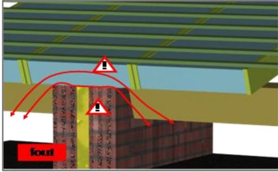
**Figure 36: Incorrect execution: installation of the roof elements across the party wall eliminates the cold bridge, but significant sound transmission occurs via the two red arrows. The sound insulation may drop below 30 dB.**
