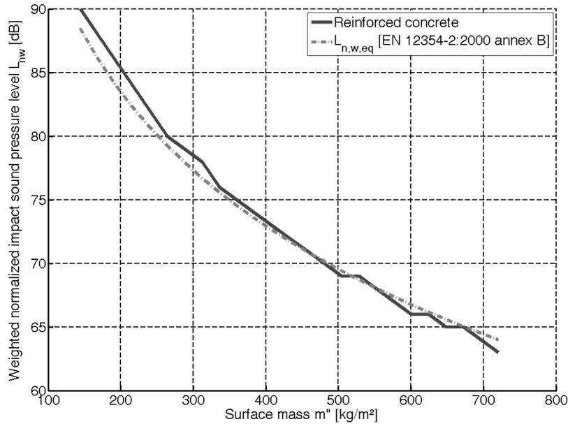
**Figure 19: Comparison of calculated results to the approximation as suggested in (NBN EN ISO 12354-2, 2000).  $L_{n,w,eq}$  refers to (NBN EN ISO 717-2, 1996) and to the bare concrete floors**
