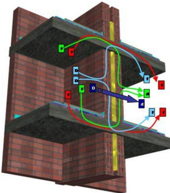
**Figure 28: The various airborne sound transmission paths to the adjacent apartment**
