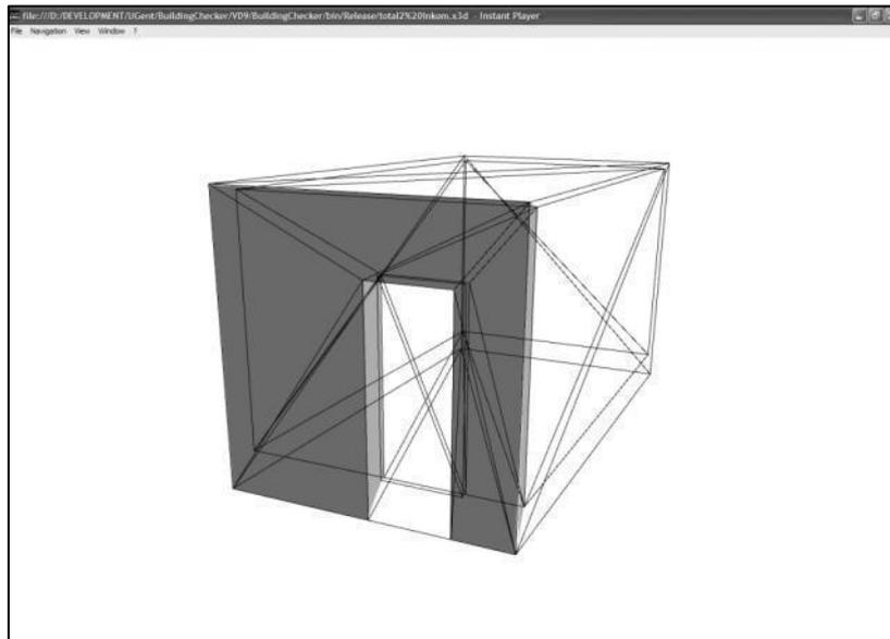
**Figure 5: The inflated mesh, representing the external geometry for a *IfcSpace* instance**
