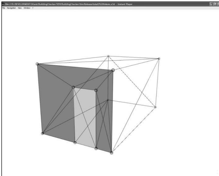
**Figure 4: The closed and directed triangulated mesh, representing the internal geometry**
