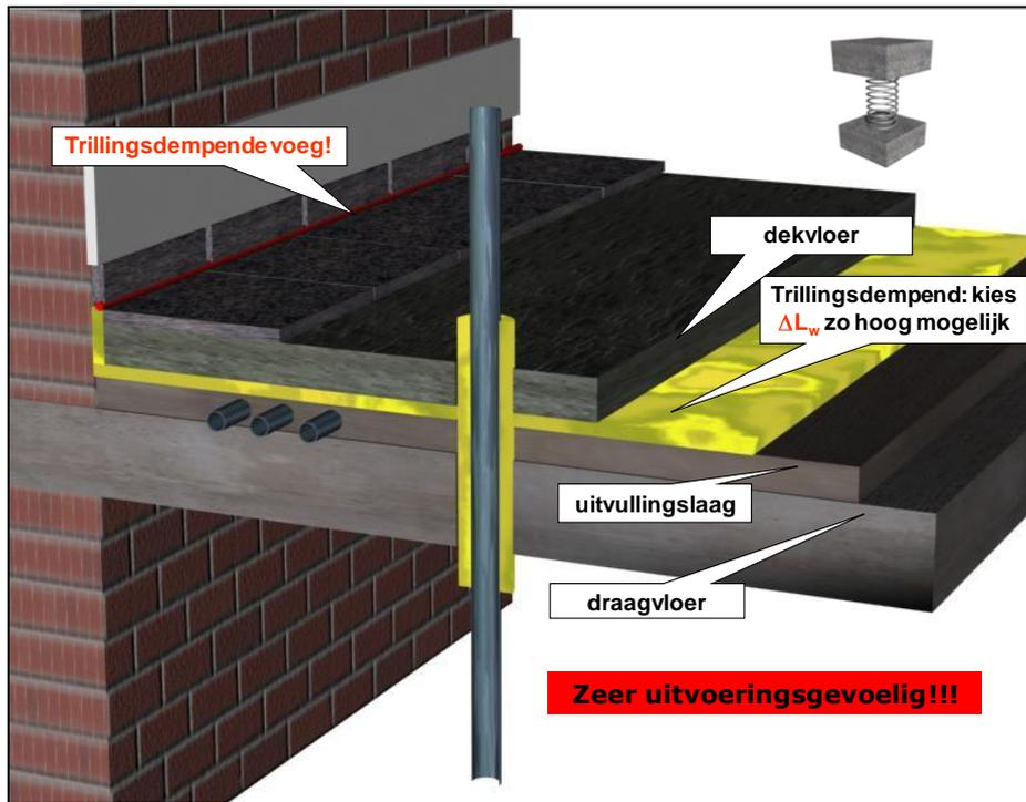
**Figure 44: Structure of a traditional floating floor**
