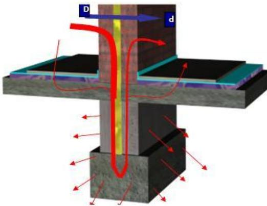
**Figure 31: Structural sound transmission through the foundations in structural building concepts based upon the construction principle involving cavity walls without ties**
