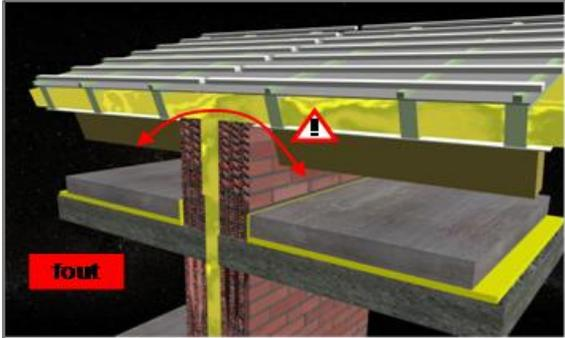
**Figure 34: Leakage sound in an incorrectly executed arrangement**
