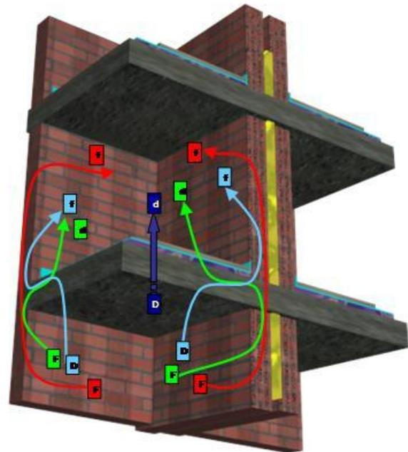
**Figure 29: The various airborne sound transmission paths to the apartment above**
