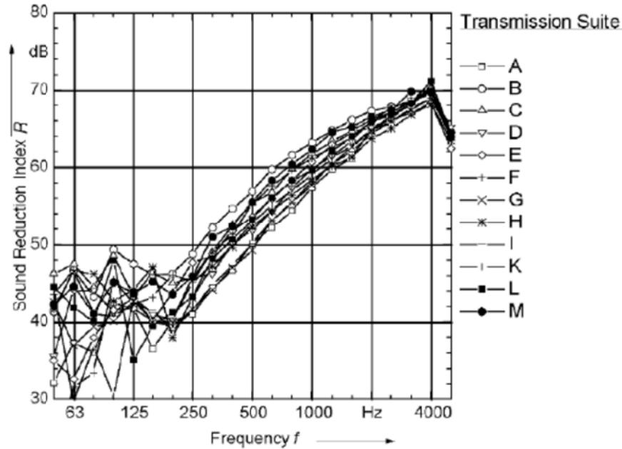
**Figure 15: The Sound Reduction Index of a similar wall in 12 different transmission suites with rigid connections (PTB comparison measurements)**
