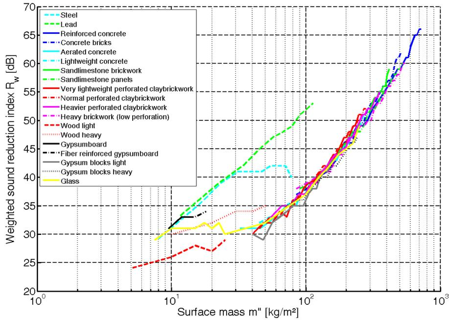
**Figure 17:  $R_w$  values as derived from the octave predictions**
