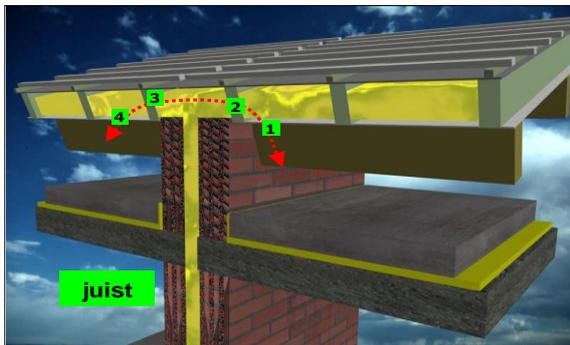
**Figure 35: Schematic diagram of correct execution: by installation of the spars/rafters against the party wall leaves, the leakage sound through 4 barriers becomes negligible**
