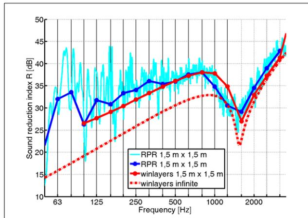
**Figure 14: Sound Reduction Index between two rooms with a baffled glass pane of dimensions 1.5x1.5 m<sup>2</sup>. The results are presented in narrow bands and in the regular third octave bands (blue line) / (the red line concerns infinite plate model, the full red line concerns adaptations to finite dimensions [calculation results by Arne Dijckmans, Laboratory of Building Physics, K.U.Leuven]).**
