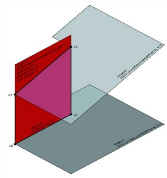
**Figure 3: The intersection of the extruded surface of the wall with the slab curve defines the wall curve**
