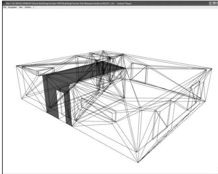
**Figure 6: Collection of closed, directed, interrelated and inflated IfcSpace meshes**
