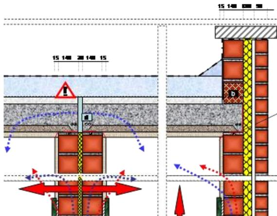
**Figure 40: The sloping roof concrete must also be interrupted**
