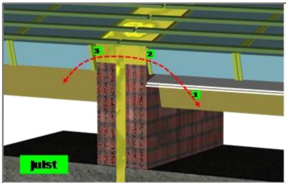
**Figure 37: Schematic diagram of correct execution for normal acoustic comfort: the roof elements are installed against the party wall leaves**
