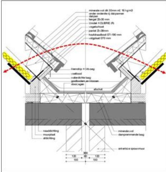
**Figure 39: Schematic diagram of correct acoustic execution: detail at the party wall of roofs sloping towards each other constructed by means of lightweight roof elements**
