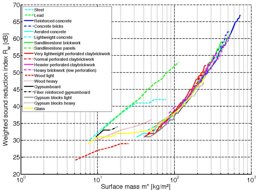
Figure 16:  $R_w$  values as derived from the third octave predictions in the function of the surface mass
