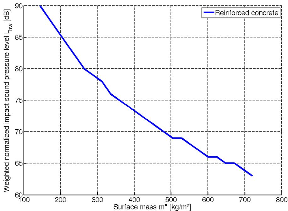
**Figure 18:  $L_{nw}$  values as derived from the third octave predictions**
