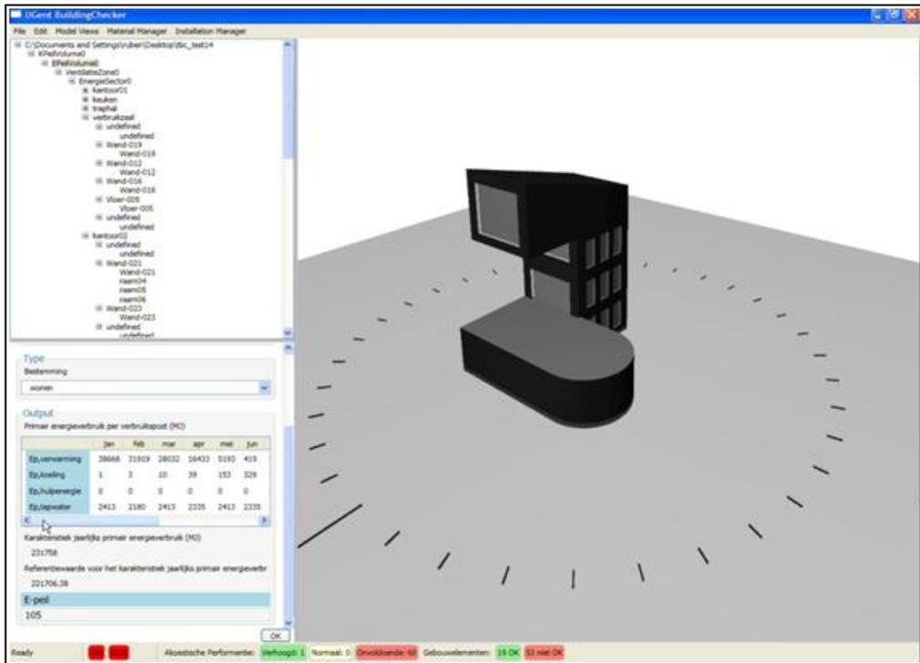
Figure 11: Tiatab BuildingChecker application, energy view with results
