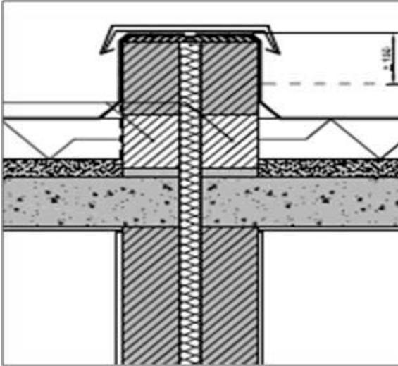
**Figure 41: Alternative involving breaking-up of the water dispersal areas at a cavity wall without ties**
