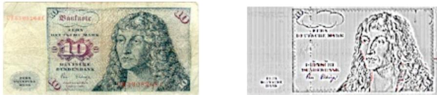
**Figure 7: Optical and Magnetic images of an old 10 DM banknote**
