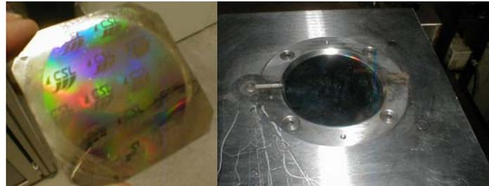
**Figure 40: “Test” Ni-master and insert in the injection mold**
