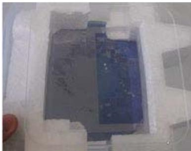
**Figure 58: Resulting silicone wafer Ni Shim separation**
