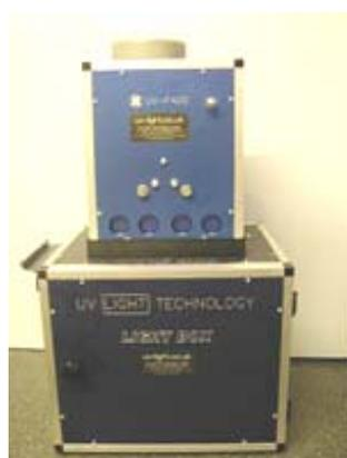
**Figure 28: UV-400 lamp system for photolithography.**
