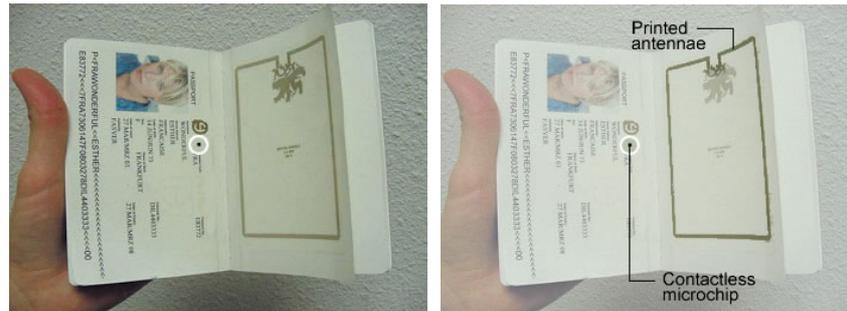
**Figure 12: Embedded RFID transponder in a passport**
