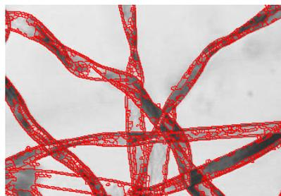
**Figure 116: Example fiber image segmentation result (microscope)**
