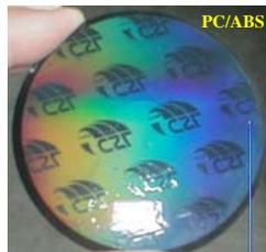
**Figure 41: Replication by direct injection molding (PC/ABS)**
