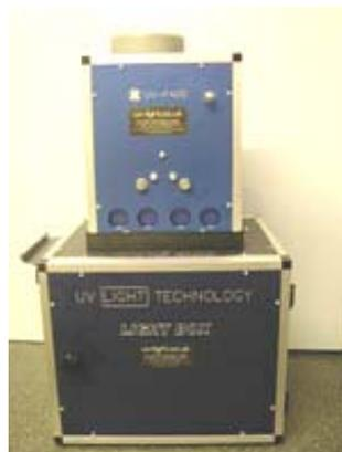
**Figure 28: UV-400 lamp system for photolithography.**
