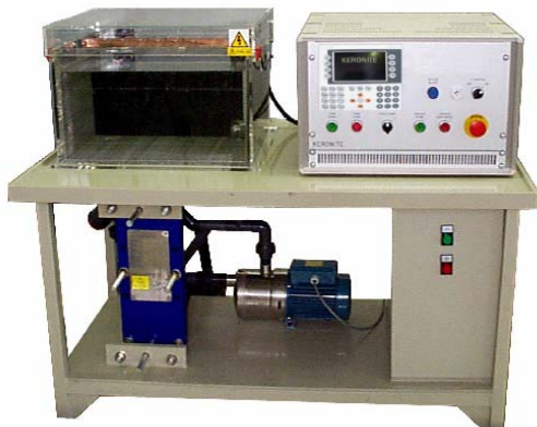
Figure 4: 10 kW laboratory equipment for the production of PEO coatings
