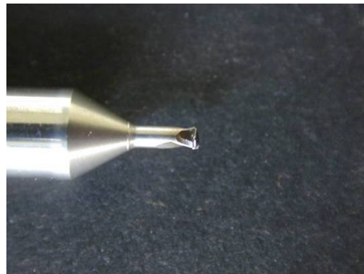
Figure 37: drill geometry for hole drilling stress measurements.
