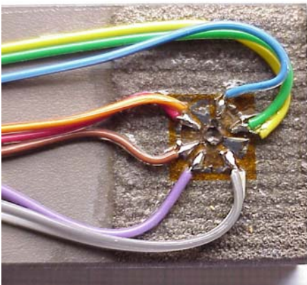
Figure 36: set up of hole drilling experiment.
