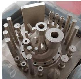
Small-scale combustion chamber and injector, ArianeGroup GmbH
