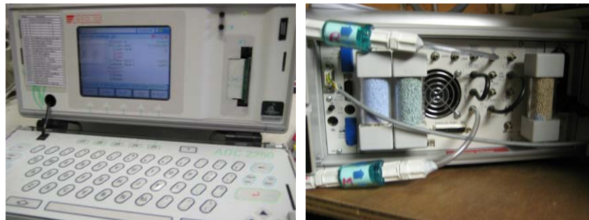
Figure 22: Stationary ADC 2250 IRGA to measure online photosynthesis and transpiration rates
