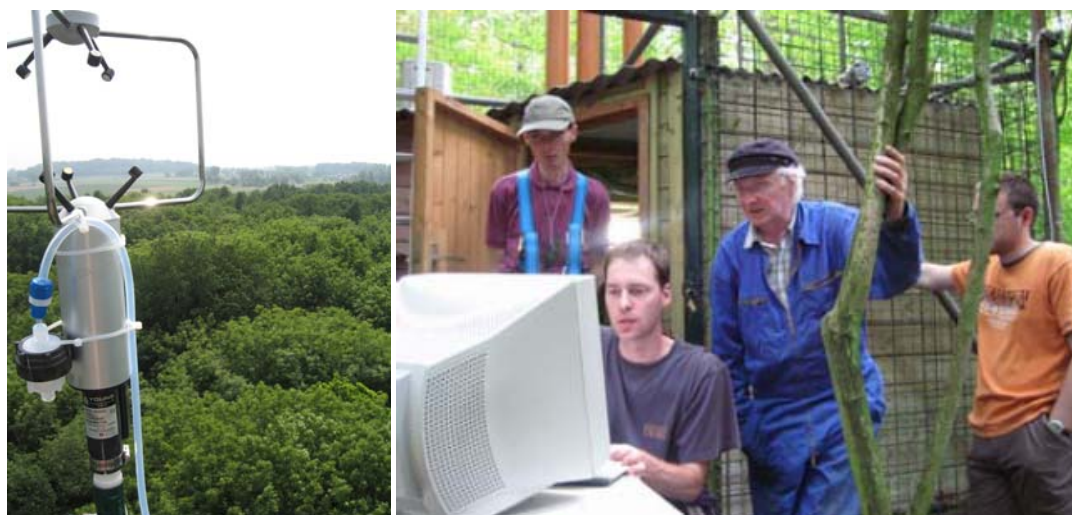
Figure 29: Left: sonic anemometer installed at the Aelmoeseneie forest. Right: logging of EC-BVOC data.
