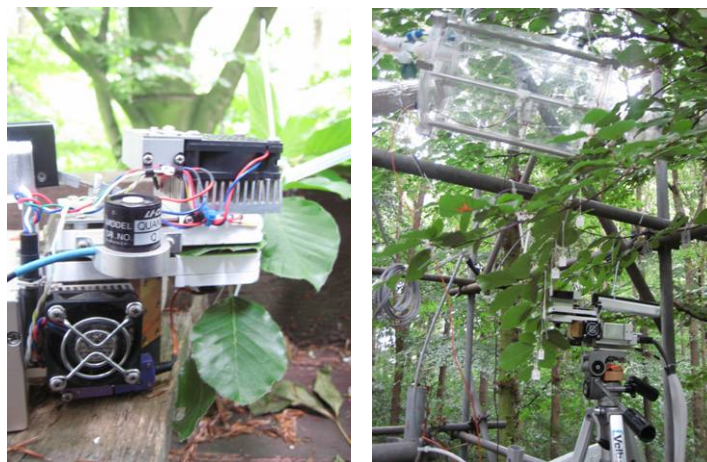
Figure 23: Portable LI-6400 IRGA in the Aelmoeseneie forest (9 July 2008) to measure offline photosynthesis and transpiration rates
