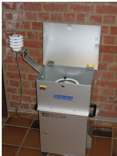
Figure 7 : High flow rate pump for environmental sampling
