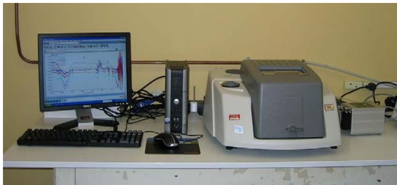
Figure 8 : Nicolet 380 FTIR spectrophotometer with peristaltic pump
