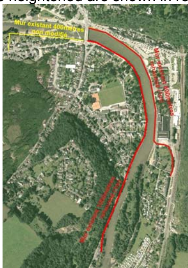
Figure 14: Situation of the permanent/mobile wall for the Ourthe
