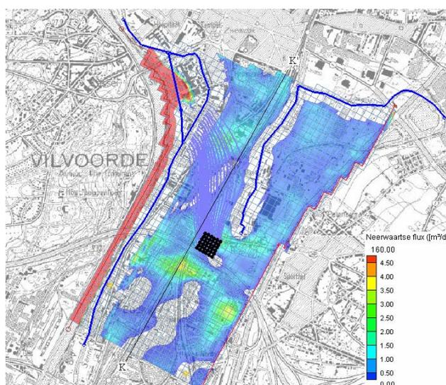
**Figure 4: Advective transport of pollutants simulated with MODPATH coming from the SRI/BIOLUX-site (colors are providing groundwater fluxes in m<sup>3</sup>/day)**
