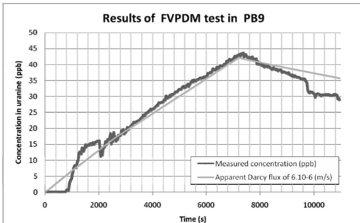
Figure 22: Results of FVPDM test performed in PB9
