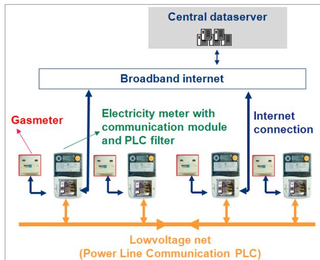
Figure 6: Eandis’ PLC based smart meter communication concept
