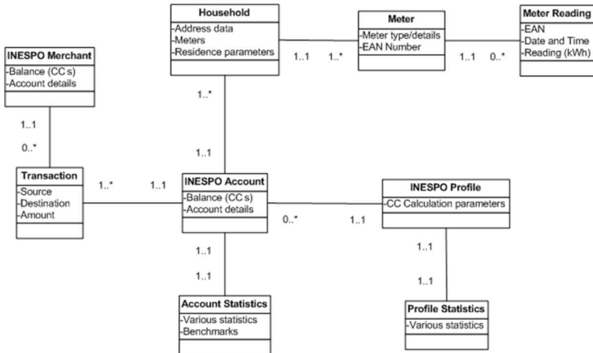
Figure 13 Back-office database class diagram
