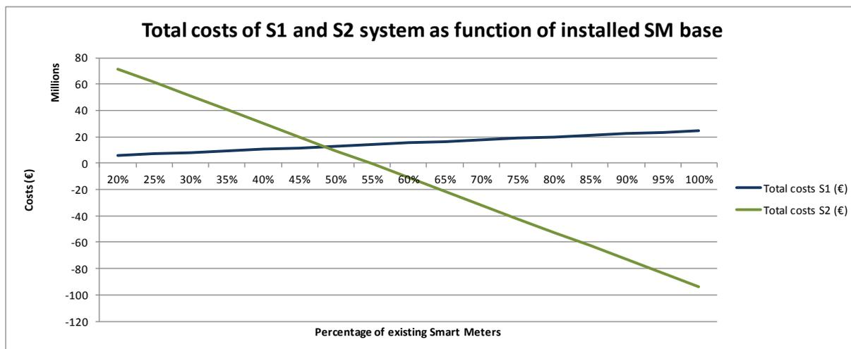
Figure 33: Costs of S1 and S2 taking into account a partial deployment of Smart Meters
