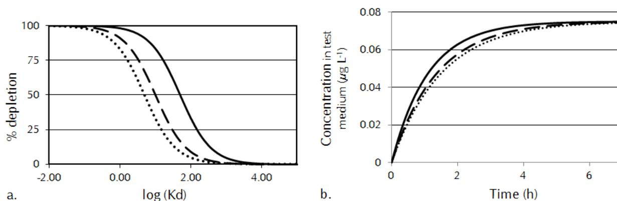
Figure 16. (a) Relation between % of depletion of the passive sampler and  $\text{Log}(K_d)$  of the absorbed compound, volume of the test medium was assumed to be 0.05L, the amount of sampler added was 1g (solid line), 5g (dashed line) or 10g (dotted line); (b) release kinetics of compounds with varying  $\text{Log}(K_d)$ : fluorene (solid line;  $\text{log}(K_d) = 3.82$ ), fluoranthene (dashed line;  $\text{log}(K_d) = 4.69$ ), benzo(a)pyrene (dotted line;  $\text{log}(K_d) = 5.56$ ).
