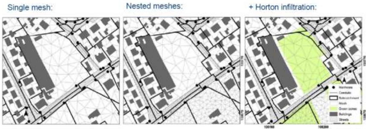
1D-2D dual drainage approach, with different mesh sizes tested and including Horton infiltration in green zones
