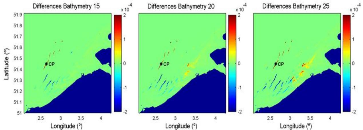
Figure 3.4-8. Differences in dissipation due to surf breaking ( $\text{m}^2/\text{s}$ ) in the original fine-scale bathymetry grid and in the adapted bathymetries (15, 20 and 25 m) from November 25, 2005 at 0h.
