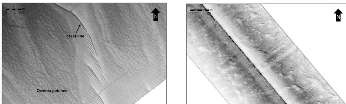
Figure 3.2-4. (left) Detailed shaded relief map of an area with very large dunes; in the troughs extensive fields of *O. fusiformis* are present (rectangle on Fig. 3.2-3); and (right) detailed side-scan sonar mosaic, showing individual *Owenia* patches.
