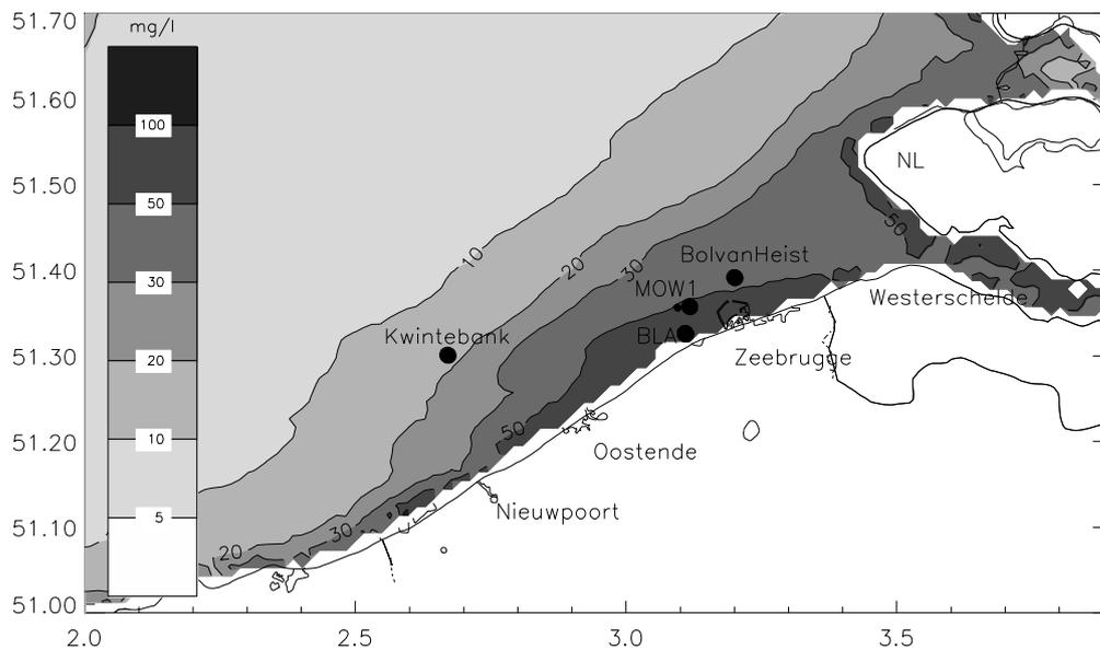
Figure 2.2-1: Map of the Belgian part of the North Sea with the in-situ measurement stations Blankenberge (BLA), MOW1 and Kwintebank and the wave measurement station Bol van Heist. The background consists of the yearly averaged surface SPM concentration (mg/l) from MODIS images (2003-2008). Coordinates are in latitude ( $^{\circ}$ N) and longitude ( $^{\circ}$ E).
