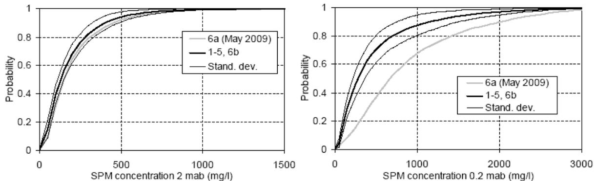
Figure 3.3-12. Cumulative probability distribution of SPM concentration measured at 2 mab and 0.2 mab. The black line (1 to 5, 6b) shows the data during the non-disposal periods  $\pm$  one standard deviation (thin black lines); the grey line shows the distributions during the dredging experiment (6a). This shows that continuous disposal results in a long-term increase of SPM concentration near the bed.
