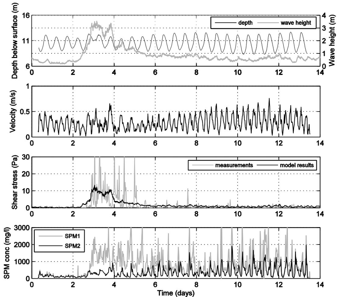
Figure 3.2-1. MOW1 site, tripod measurements of 22 November – 5 December 2005 (survey 2005/29). From up to down: depth below water surface (m) and significant wave heights; ADV current velocity (m/s); shear stress (Pa) derived from the ADV and from the hydrodynamic model and SPM concentration at 0.3 mab (SPM1) and 1.9 mab (SPM2).
