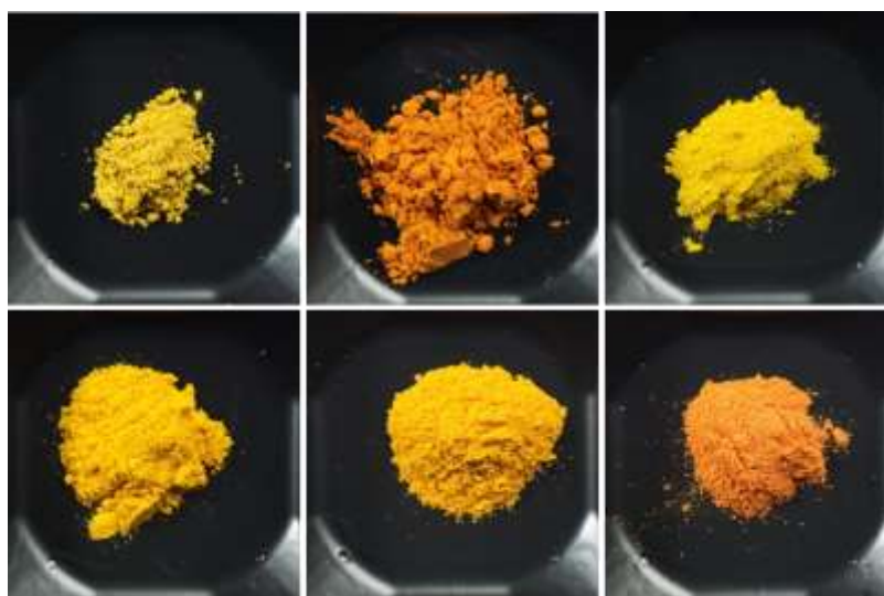
Figure 12. Photographs of (a) ground natural orpiment, (b) ground natural realgar, (c) ground g\text{-As}_{25}\text{S}_{75} , (d) g\text{-As}_{30}\text{S}_{70} , (e) g\text{-As}_{34}\text{S}_{66} and (f) g\text{-As}_{40}\text{S}_{60} .
