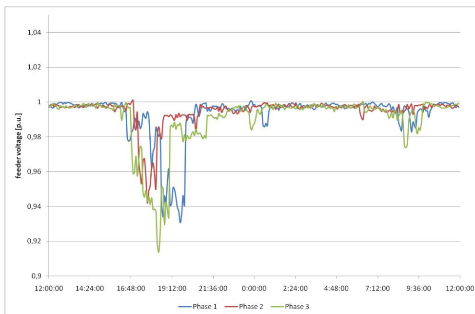
Figure 2: Voltage drop at the end of a feeder when electrical vehicles are present.
