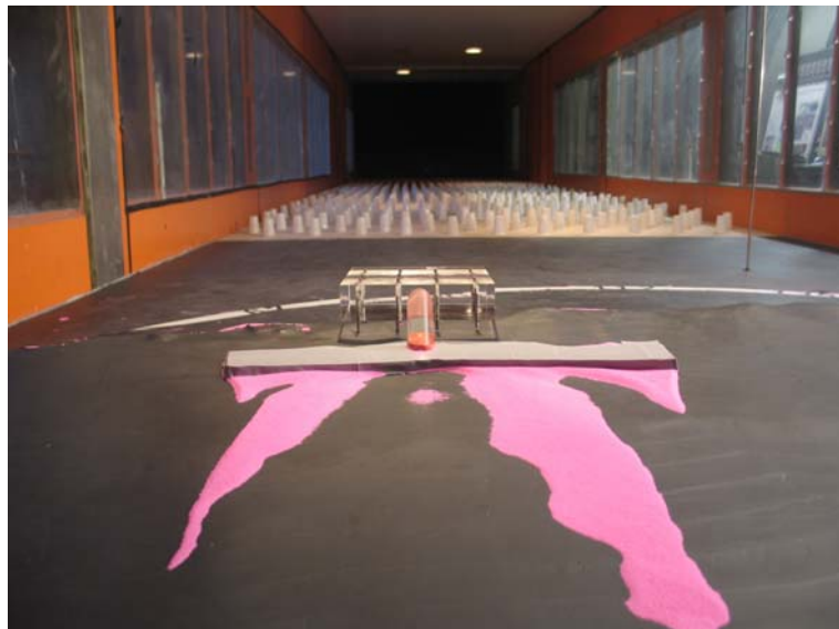
Fig. 2.26: WTT-3: Sand erosion testing with garage building integrated.
