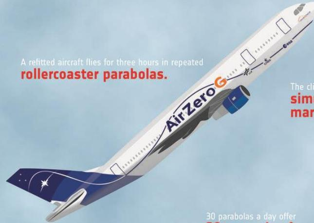
30 parabolas a day offer **20 seconds of microgravity** each time.
